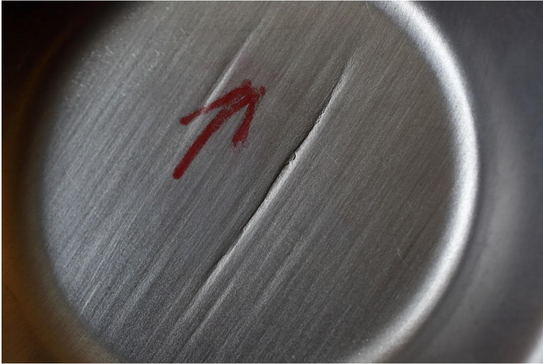
Figure 8 Roping and multiple local necks observed at the bottom side of a Marciniak-Kuczynski sample [19].
