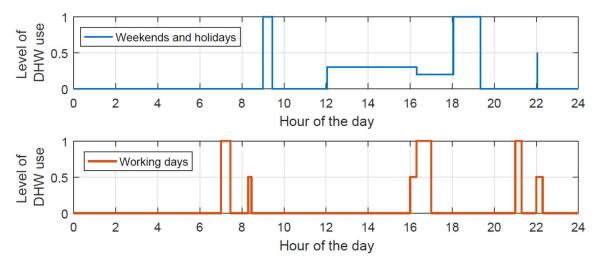
Fig. 3. Domestic hot tap water use profiles based on the standard values
