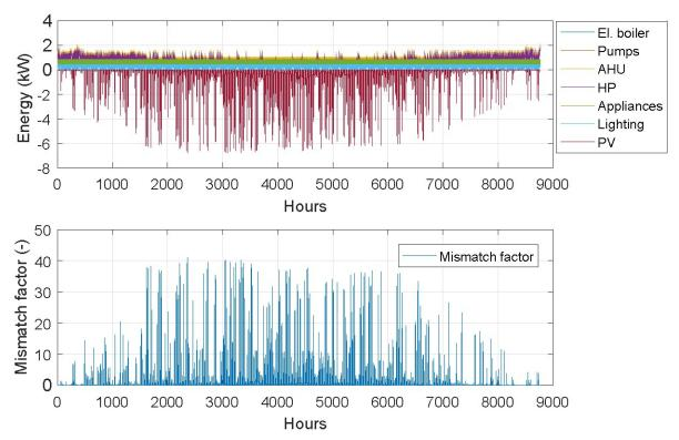
Fig. 14. Electricity use, electricity production, and mismatch factor for reference model
