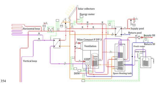
Fig. 7. Heating and cooling system with solar thermal system, GSHP and EAHP
