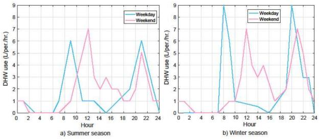
Fig. 2. DHW profile for four occupants in the residential building stock under two seasons
