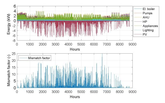
Fig. 15. Electricity use, electricity production, and mismatch factor for OB model
