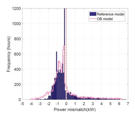
Fig. 16. Histogram of the power mismatch when the occupant behavior was treated
