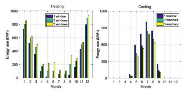
Fig. 13. Heating and cooling energy use depending on number of opened windows simultaneously
