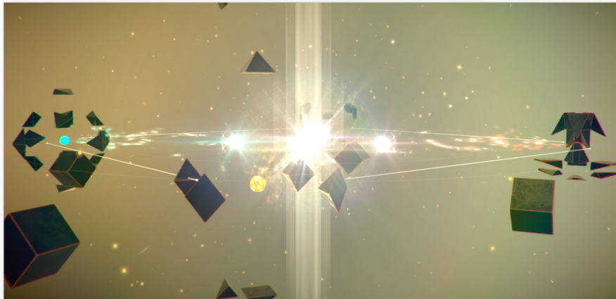
Figure 9.3 | Objects placed in the edges of the VR environment can get blurry
