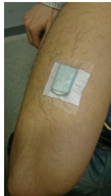
(d) Accelerometer attached using adhesive film. Position above knee slightly higher than during collection.
