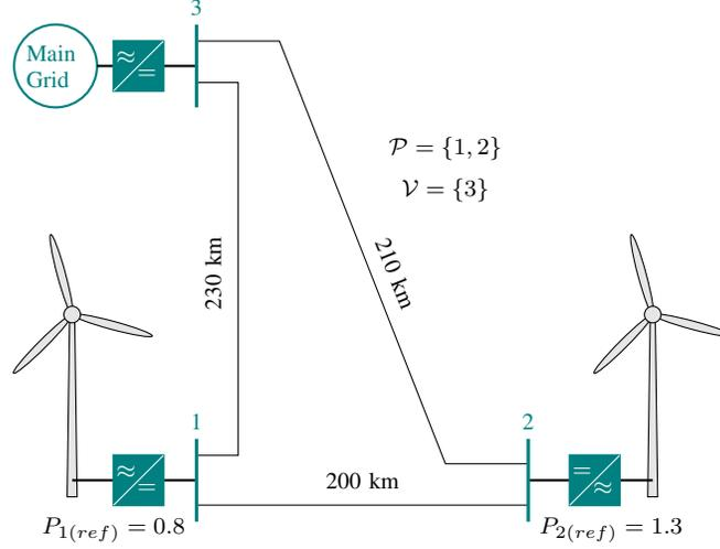
Fig. 1. Example of a simple MT-HVDC grid with two offshore wind farms
