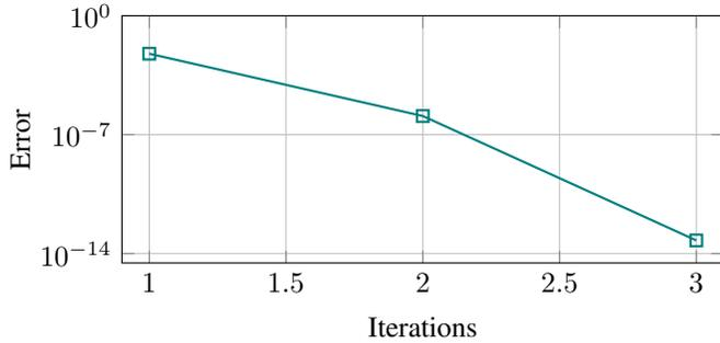
Fig. 5. Superconvergence of Newton's method applied to a reduced CIGRE bipolar DC grid test system from an initial point  $v_k = 1$
