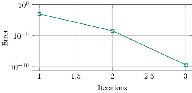
Fig. 3. Super-convergence of Newton's method applied to a simple MT-HVDC grid from an initial point  $V_P = (1.00, 1.00)^T$
