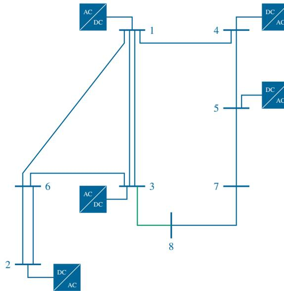
Fig. 4. Reduced CIGRE bipolar DC grid test system
