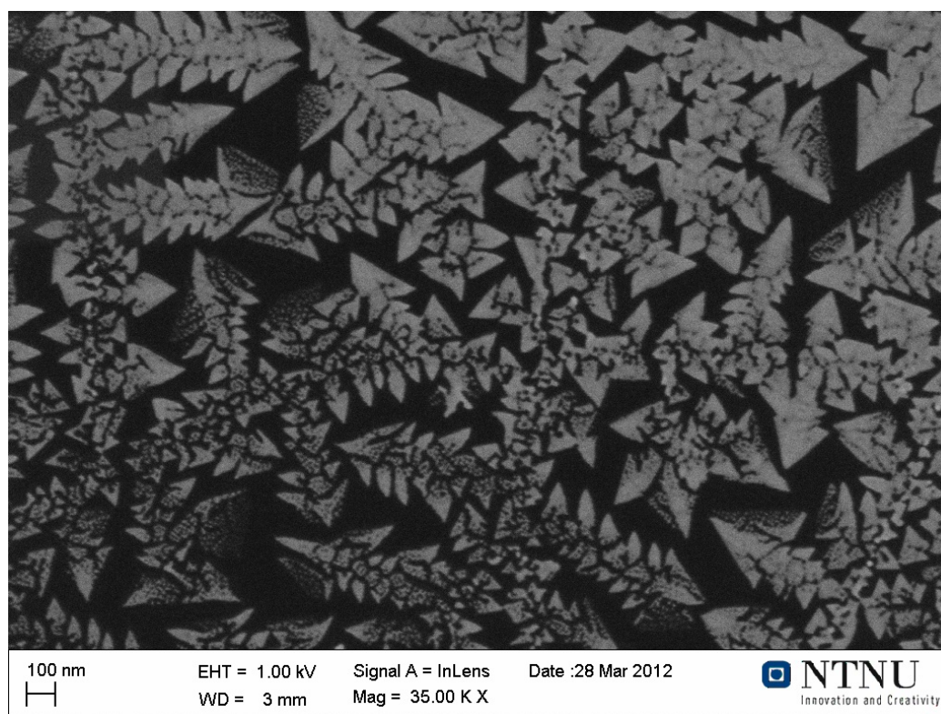
Figure 4.9: Gold nanostructures on HOPG at 10 minutes of evaporation and 9 minutes of sputtering. This SEM image shows the nano-dendrites on sample 7 after 9 minutes of sputtering. In some areas the gold has been mostly removed and what remains are gold dots, still in the shape of the dendrites. The scale can be seen in the bottom left of the image.
