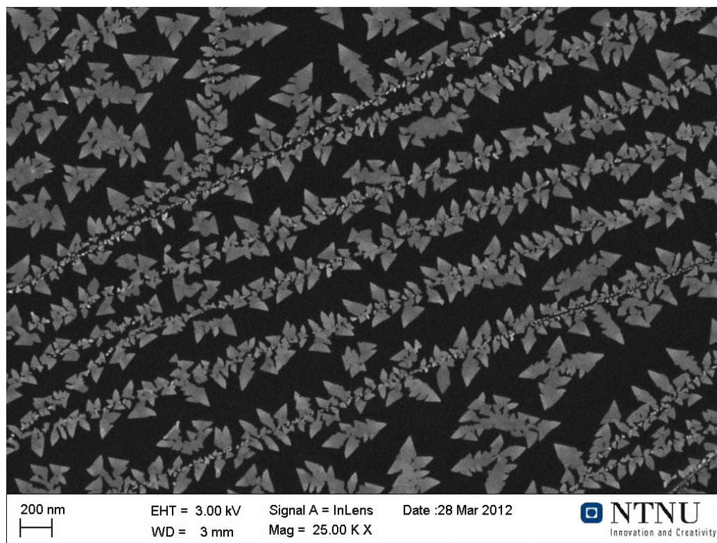
Figure 4.7: Gold nanostructures on HOPG at 3 minutes of evaporation. This SEM image from sample 9 shows nanostructures of gold evaporated onto graphite at 310 K for 3 minutes. The spaghetti-like structures and nanoislands both have complex branching, which all have a triangular shape. The scale can be seen in the bottom left of the image.
