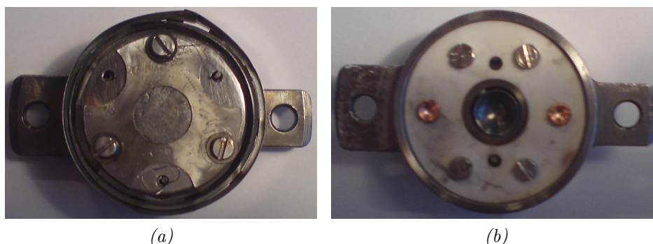
Figure 3.3: (a) show the front of the sampleholder. The thermocouple wires protrude at the bottom part of the holder. (b) show the connections on the back of the sample holders. As the holder is seen in (b) the top two connections are for the thermocouple, the middle two are for the heating filament and the bottom two are for grounding. In (b) the sample holder is rotated such that the top part is directly behind the lower part of (a)
