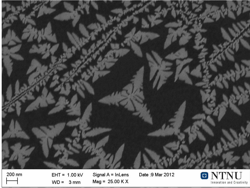
Figure 4.1: Gold nano-dendrite on HOPG. This SEM image from sample 3 shows the dendritic and spaghetti-like nanostructures of gold evaporated onto graphite at 310 K for 25 minutes. The scale can be found in the bottom left of the image.
