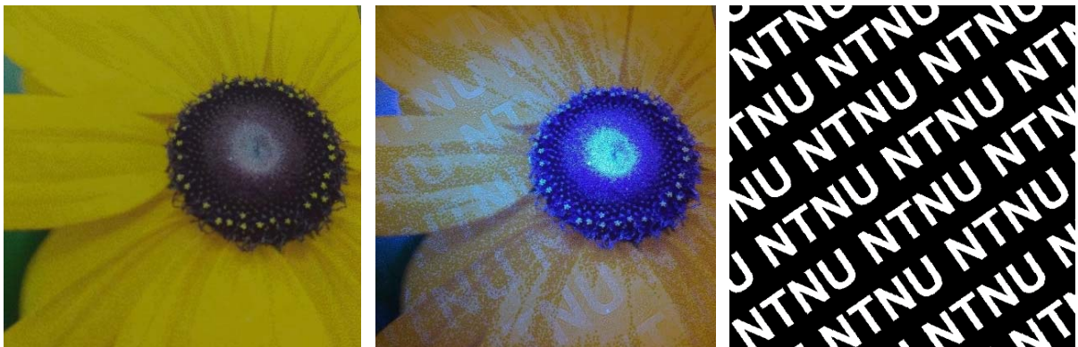
Figure 3. Printout as seen under room illumination (left) and the identical printout when a UV light is added (middle). The embedded CDBS-WM binary pattern is shown on the right.
