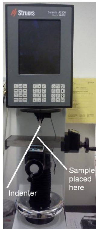
Figure 3.6: The Struers Duramin A-2500 used for hardness measurements.
