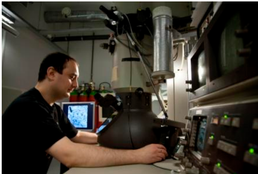
Figure 2.8: A Philips CM30 TEM operated by my supervisor Calin D. Marioara. Notice the vertical column where all the important components are placed.
