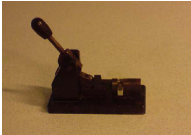
Figure 3.8: Device used to make 3 mm discs.
