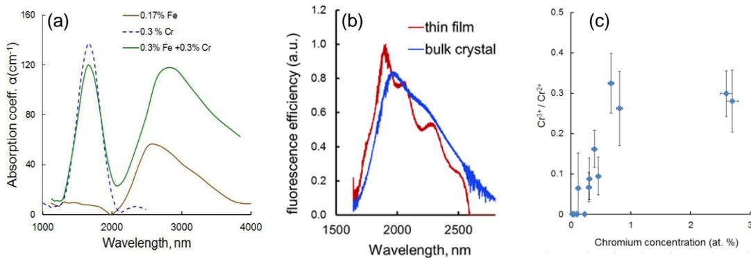
Fig. 1 Optical properties of TM-doped ZnS films (a) absorption coefficient of 4  $\mu\text{m}$  thick films with 0.17% Fe, 0.3% Cr, and 0.3% of both Fe and Cr, showing isolation of the peaks (b) fluorescence of Cr:ZnS film, compared to bulk sample, normalized by the sample absorption. Oscillations in film data are interference effects. (c) Ratio of  $\text{Cr}^{3+}$  to  $\text{Cr}^{2+}$  as a function of Cr concentration.
