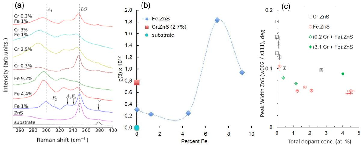
Fig. 2 (a) Raman spectrum of the films studied, showing modes in both spectra associated with substitutional transition metal ions. For Fe, good order is maintained for >4% concentration. (b)  $\chi^{(3)}$  derived from optical Kerr effect measurements. Dashed line is a guide to the eye. (c) X-ray diffraction full width half maximum vs concentration for Cr and Fe substitutions in the lattice.
