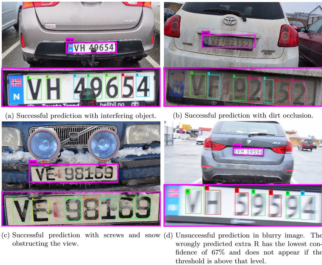
Figure 6.7: Examples of plate detection and character detection by the final system in challenging conditions.
