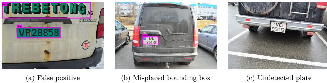
Figure 6.1: The three mistakes done by the plate network in the first iteration
