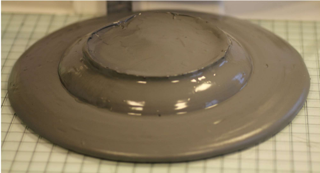
Figure 3. Final shape laboratory quickness test (height 40 mm, diameter 237 mm), Heimdal clay, remolded shear strength c_{ur} = 0.2 kPa (Photo: Thakur, V.)
