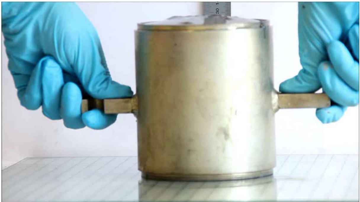
Figure 1. Cylinder (internal height 120 mm, diameter 100 mm) filled with remolded sensitive clay, standing on glass plate. (Photo: Thakur, V.)
