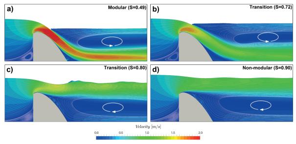
**Fig. 4** Velocity contours with streamlines for the four different types of submerged flow conditions: a) modular flow with submerged hydraulic jump (S = 0.49); b) transition with detached jet and submerged hydraulic jump (S = 0.72); c) transition with surface jet and partial hydraulic jump (S = 0.80); d) non-modular flow with surface jet (S = 0.90).
