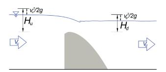
Fig. 1 Sketch of the ogee-crested weir, with the definition of the upstream and downstream total heads.
