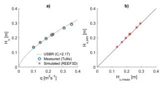
Fig. 2 a) Comparison of theoretical, measured and modeled head-discharge relationships; b) Comparison of modeled and measured upstream heads at different flow rates.
