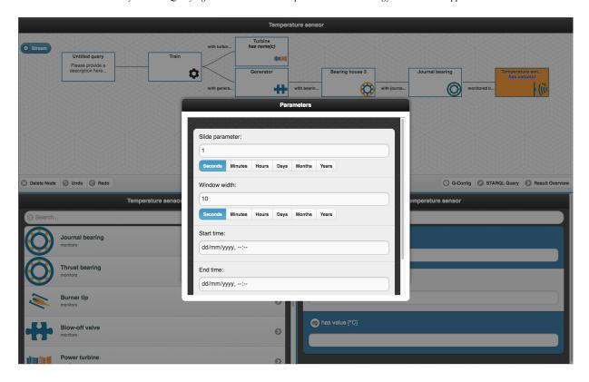
$Fig.\ 6.\ Optique VQS\ with\ stream-temporal\ querying-parameter\ selection.$
