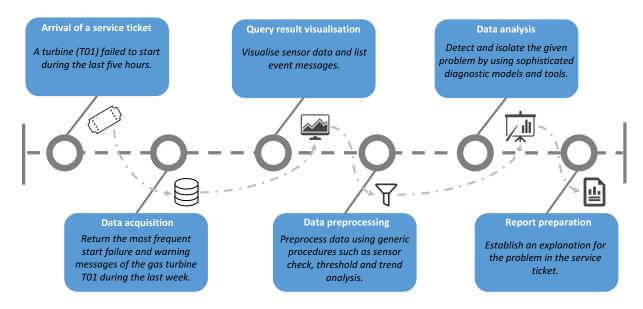
Fig. 2. Siemens service process for reactive tasks.
