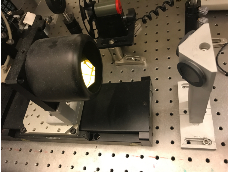
Figure 3.3: Delay line with stationary mirrors and retroreflector.
