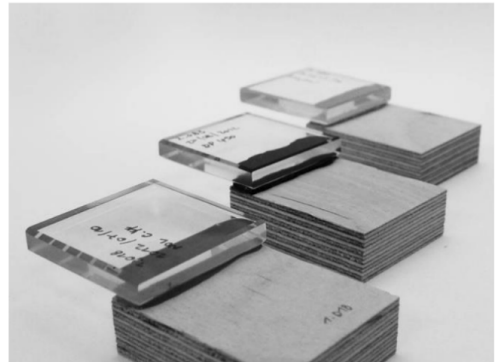
Figure 2: Dimensions of shear specimens (left) with thickness of the adhesive layer between 1 and 4 mm (values in brackets for specimens at TUD) and finished plywood-glass specimen prior to testing (right)
