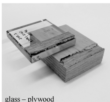
Figure 8: Typical failure pattern for DP 490 tested at room temperature: partial failure of plywood and loss of adhesion to plywood surface (left), failure of the one or more plywood layers (center), wood failure (right)
