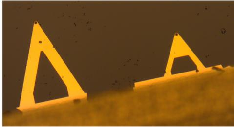
**Fig. 3.14:** A optical snapshot of the large and the small tip of a *Contact Mode* cantilever used in the lab. The geometric properties of the large and the small tip are described in Table 3.2. The dark spot at the end of each cantilever is the tip itself. The other dark spot on the cantilevers are most likely dust.
