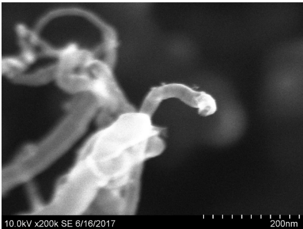
Figure F.6: S(T)EM image of W 2 C/CNT, 200 nm scale
