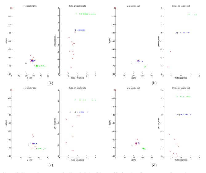
Figure 5: Estimated pipe position (y, z) to the left and bearing  $(\theta, \phi)$  to the right at x=1 meter distance from origo when the AUV is placed at four different positions along the pipeline (a = pos. 1, b = pos. 2, c = pos. 3, d = pos. 4). Estimations are based on the stereo vision approach (red), the echo sounder in combination with left (blue) and right (green) camera. Ground truth is indicated by a black circle, and origo is indicated by a red circle.
