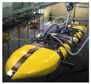
Figure 3: The AUV is a vehicle developed for research purposes, with a sensor package including two color cameras, echo sounder, sonar and an inertial measurement unit (IMU). A GPS mounted on an antenna on the AUV is available for test purposes and position verification while operating the AUV near the surface.
