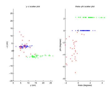
Figure 6: Deviations from the ground truth in estimated pipe position (y, z) to the left, and pipe angle  $(\theta, \phi)$  to the right, in a plane at x = 1 meter. Stereo vision results in red, echo sounder combined with left camera results in blue and echo sounder combined with right camera results in green. Ground truth indicated by a black circle in origo.
