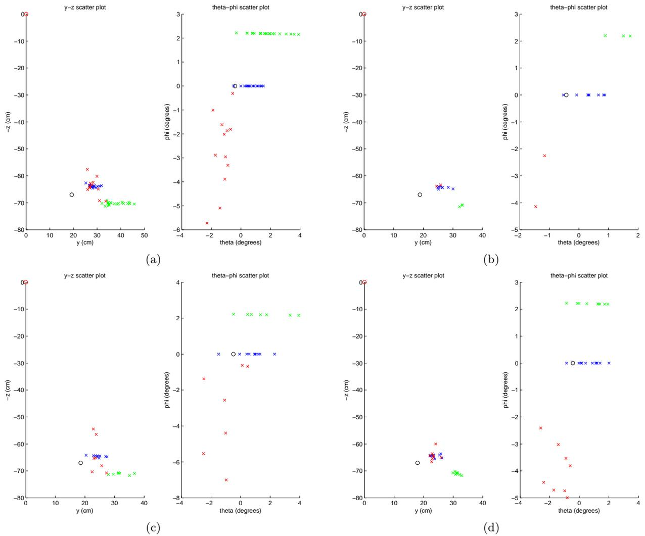
Figure 5: Estimated pipe position ( $y, z$ ) to the left and bearing ( $\theta, \phi$ ) to the right at  $x=1$  meter distance from origo when the AUV is placed at four different positions along the pipeline (a = pos. 1, b = pos. 2, c = pos. 3, d = pos. 4). Estimations are based on the stereo vision approach (red), the echo sounder in combination with left (blue) and right (green) camera. Ground truth is indicated by a black circle, and origo is indicated by a red circle.
