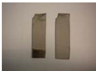
Fig 1. A brown layer could clearly be observed on the cathode (left electrode)
