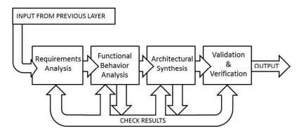
Figure 8. Model-based systems engineering process [87].
