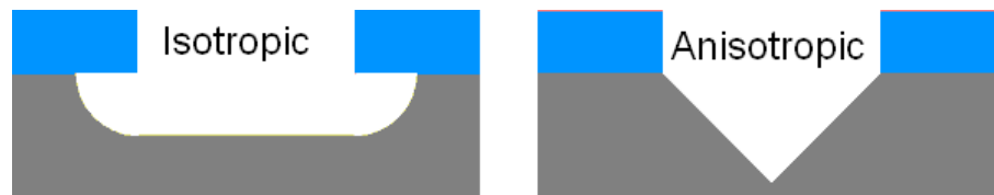
Figure 4.2: Isotropic vs anisotropic etching profiles. Blue is etch mask, grey is the substrate
