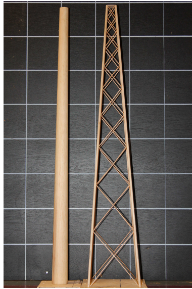
Figure 3.1: Monopile (left) and the truss tower (right)
