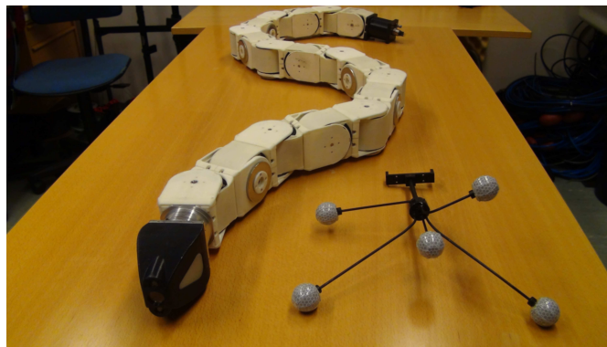
Figure B.1: The snake robot Mamba and the marker attachment for the motion capture system.
