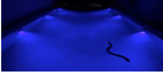
Figure 6.3: The snake robot Mamba in the MC-lab. The basin is equipped with six motion capture cameras, three mounted on each side.
