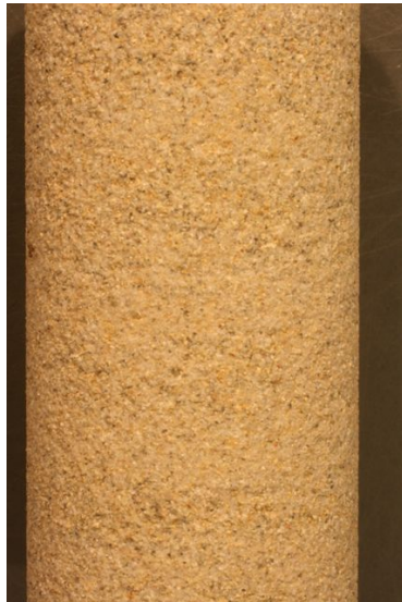
Figure 16: Castlegate surface without epoxy.
