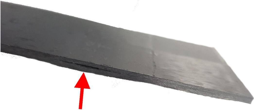
Figure 82: Defect found in one of the compression samples.
