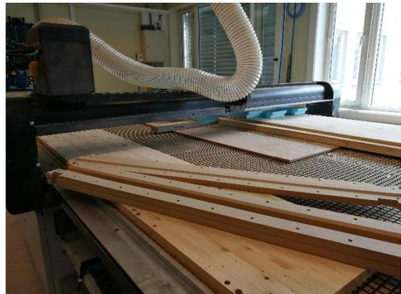
Figure 64: Mould in the milling machine
