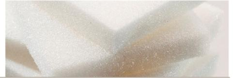
ROHACELL® IG and ROHACELL® IG-F products are closed-cell rigid foams based on polymethacrylimide (PMI) chemistry, which do not contain any CFC's.
