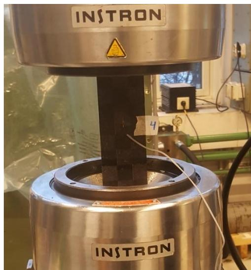
Figure 29: Experimental setup for tension testing
