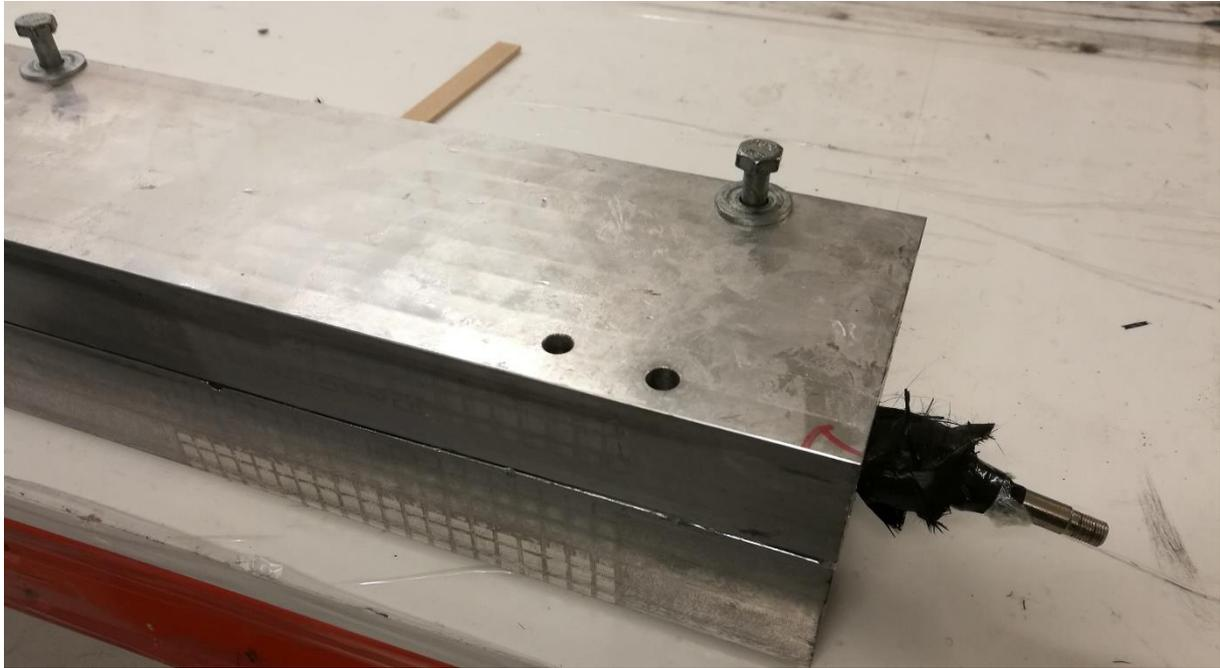
Figure 40: Mould after lay-up with bicycle tube and valve
