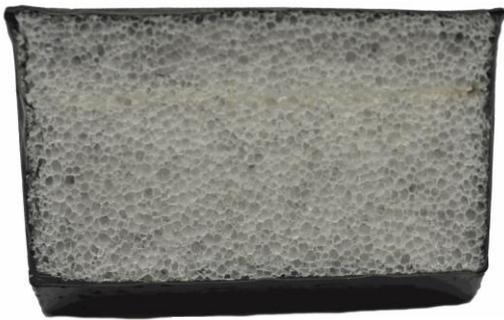
Figure 92: Cross section of compression moulded sample
