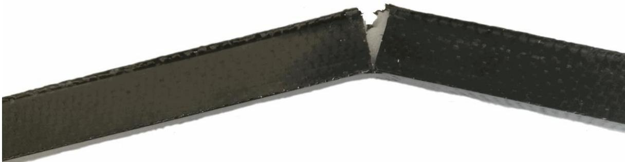
Figure 79: Failure mode of sample 4
