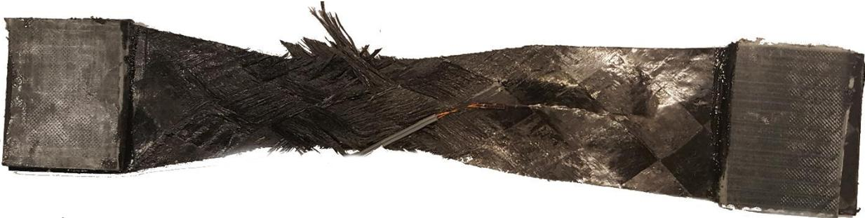
Figure 81: Failure mode for shear samples
