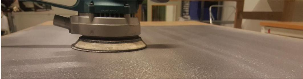
Figure 24: Sanding to remove surface scratches
