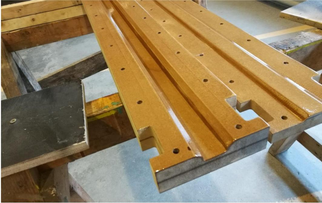
Figure 65: Surface finish after two component clear coat
