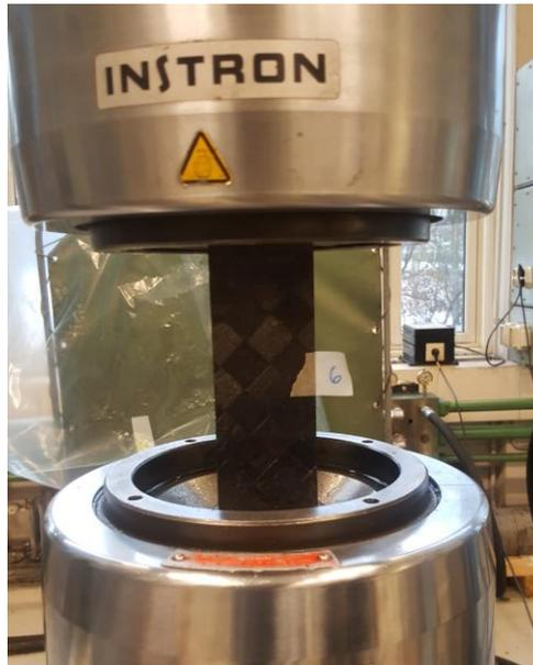
Figure 30: Experimental setup for shear testing
