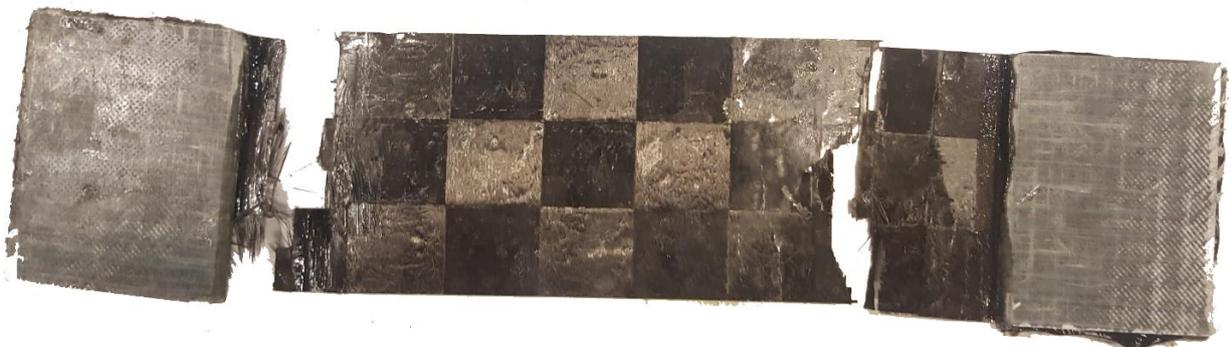
Figure 80: Typical tension specimen failure
