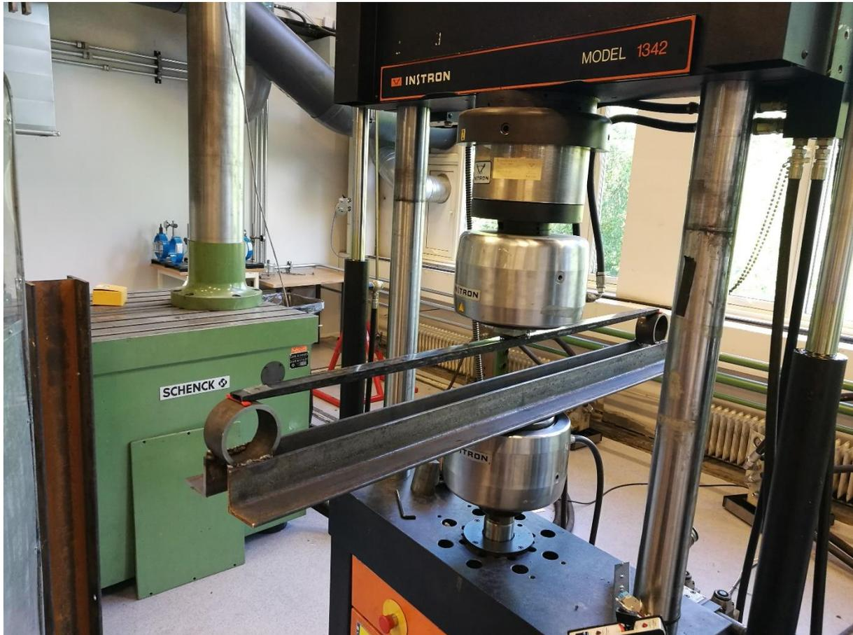
Figure 77: Test setup for testing the spar
