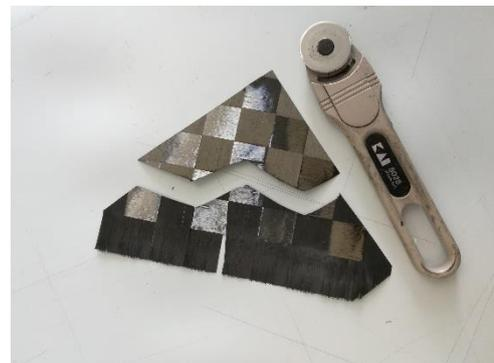
Figure 34: The anti-flaring properties of textreme
