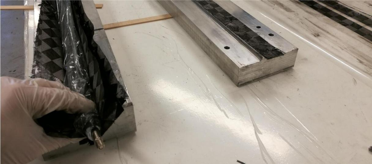
Figure 39: The bladder in the mould
