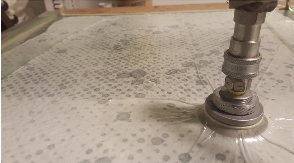
Figure 25: Curing of laminates in room temperature
