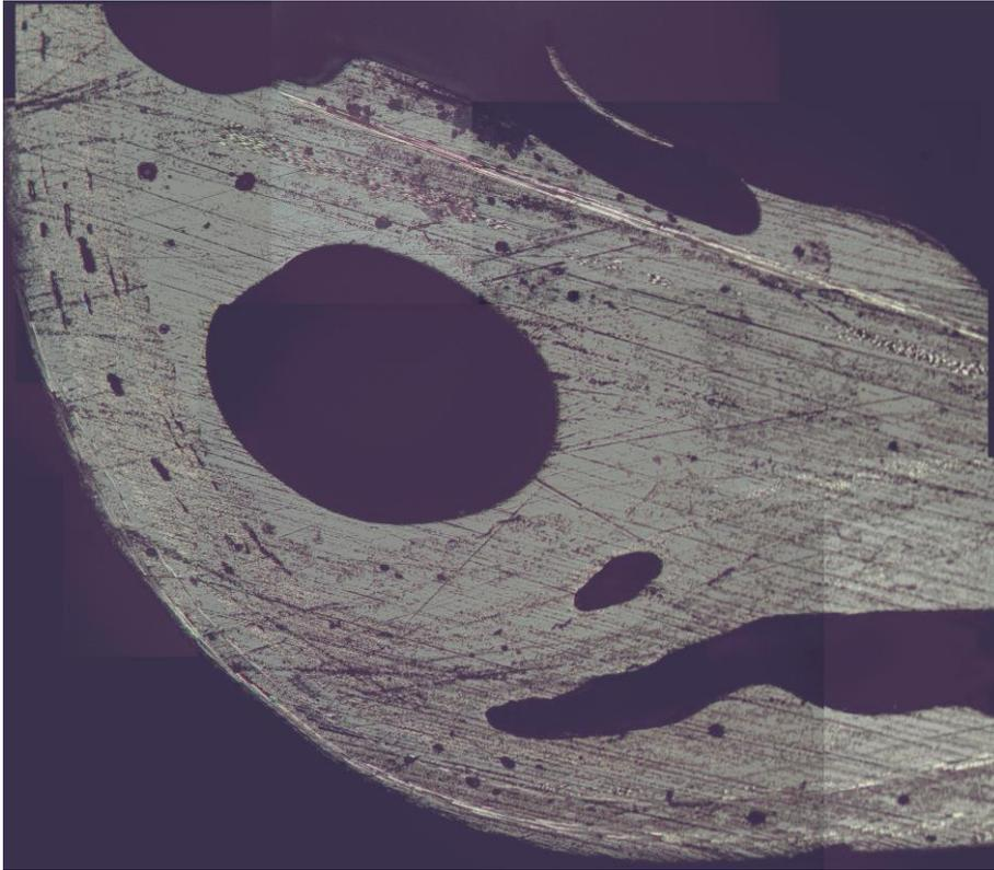
Figure 94: Cross section microscopy of the bladder moulded sample
