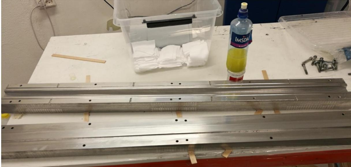
Figure 33: Process of applying release coating
