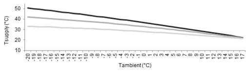
Figure 2 Heating curve. (supply temperature for space heating vs. outdoor temperature).
