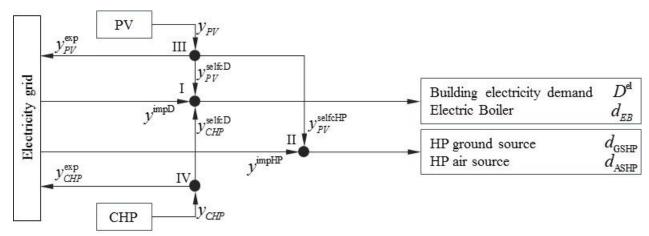
Figure 3 Graphical description of the hourly electricity balance.
