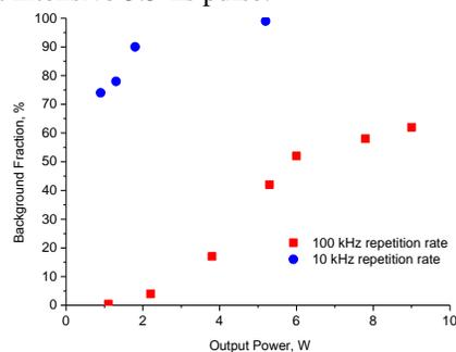
Fig. 4. Fraction of the spectral background in the total output radiation.
