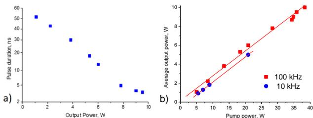
Fig. 3. Pulse compression (a) and laser efficiency (b) in the 2<sup>nd</sup> stage amplifier.
