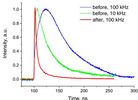
Fig. 2. Pulse shapes before and after the 2<sup>nd</sup> stage amplifier.
