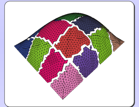
Figure showing the solution of The Poisson Equation. Each color is equivalent to one block in CUDA. The stripe is not shown
