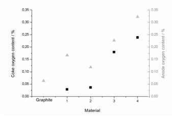
Figure 7. Total oxygen content of the cokes (black squares) and their corresponding anodes (grey triangles). Graphite is also shown for a comparison.
