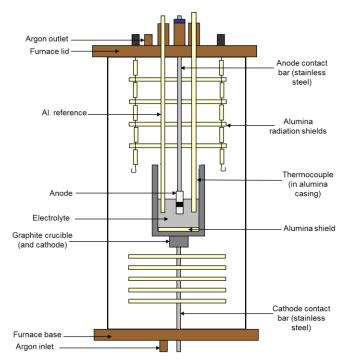
Figure 3. The furnace and crucible setup.
