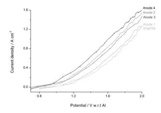
Figure 4. Polarisation curves of graphite and anodes 1 to 4 recorded at 0.1 V s<sup>-1</sup>. From left to right: Anode 4 (black), Anode 2 (medium grey), Anode 3 (dark grey), Anode 1 (grey) and graphite (light grey). Only forward scans from OCP to 2 V are shown for clarity.
