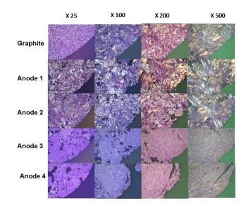
Figure 6. Optical microscopy images (under polarised light) of anodes mounted in epoxy and polished down to  $1\mu m$ .
