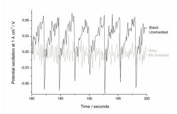
Figure 5. Potential in volts measured at a graphite anode at 1 A cm<sup>-2</sup>, normalised around zero to show oscillation. Measurements were performed with either the new BN shielding with only a vertical surface (grey), or an unshielded rod with both vertical and horizontal surfaces (black).
