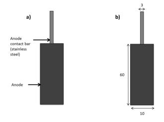
Figure 2. The anode assembly used in [15], which was also used in this study to investigate the impact of anode geometry on electrochemical measurements. When immersed 1.5 cm in the melt, this had an approximate active anode surface area of 5.5 cm<sup>2</sup>. b. with dimensions (mm)
