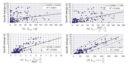
Figure 5. Correlations between specific leakage (q), hydrostatic height (h<sub>static</sub>) and input variables of Q-system based on Khimti tunnel log and injection grouting records (Panthi, 2006).
