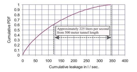
Figure 7. Calculated cumulative leakage for 1246 metre of the headrace tunnel near Adit 2 (Panthi, 2006).
