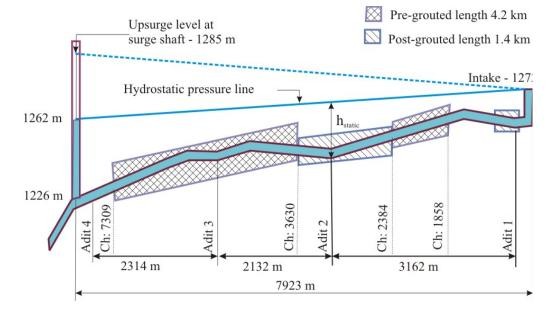
Figure 4. Khimti headrace tunnel profile showing hydrostatic pressure (h<sub>static</sub>) line during operation and areas with preinjection and post-injection grouting (Panthi, 2006). The Figure is not in true scale.
