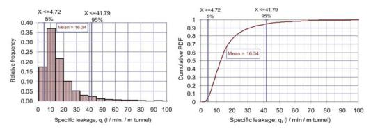
Figure 6. Distribution of specific leakage  $(q_i)$  between chainage 2384-3630, covering 1246 metre of the headrace tunnel from Adit 2 (Panthi, 2006).
