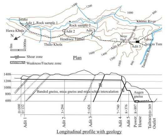
Figure 2. Project topography and profile with geological description of the waterway (Panthi, 2006).
