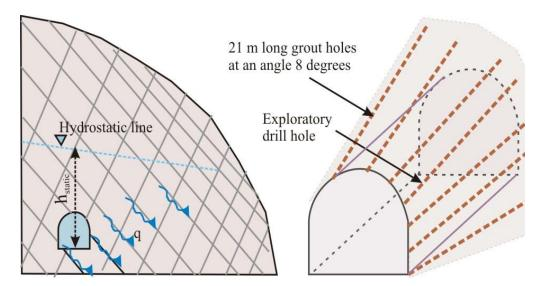
Figure 3. Principal illustration showing possible water leakage through an unlined / shotcrete lined tunnel (left), exploratory drill hole and grout/curtain for preventing water leakage (right) (Panthi, 2006).
