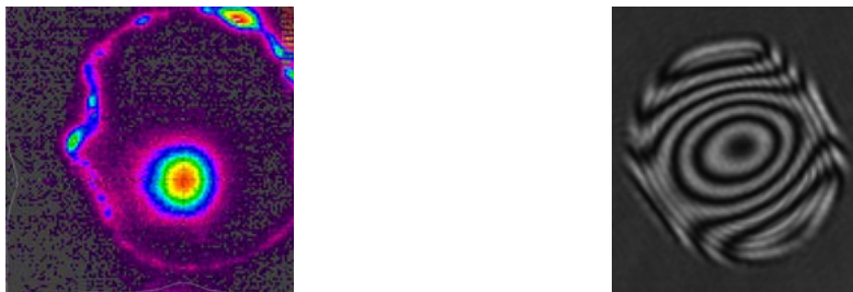
Fig. 2. Infrared picture of the pumped disk (left) and interferometry picture of the cold disk (right).
