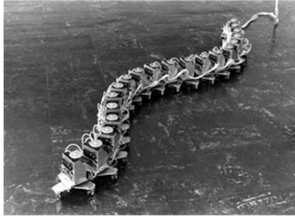
Figure 1: The snake robot ACM III , which was the world's first snake robot developed by Prof. Shigeo Hirose in 1972. Courtesy of Tokyo Institute of Technology.
