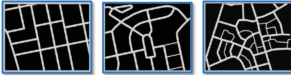
Figure 4 - Urban layouts: Orthogonal, curve and organic layout (Lahart et al., 2014)
