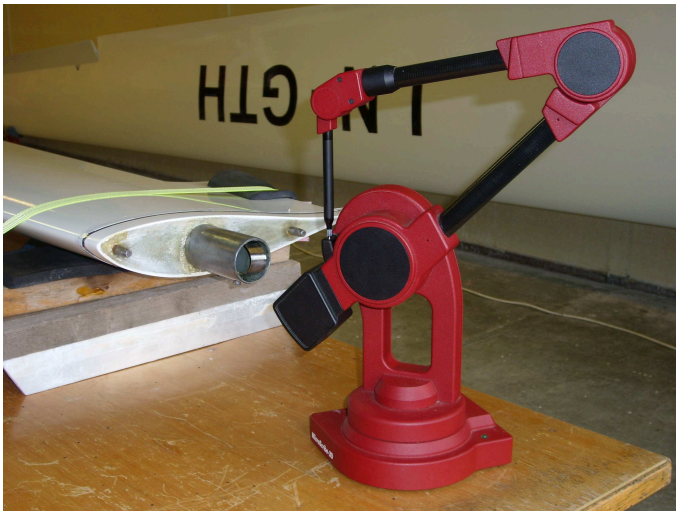
Figure 2: Microscribe digitizing arm.
