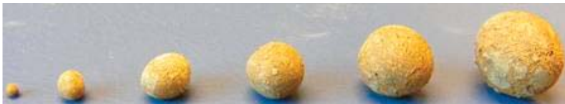
Caption Fig. 1: Illustration of LWA pellets produced in a pilot-scale rotary kiln. Diameters range from 1.8 mm (left) up to 12 mm (right).
