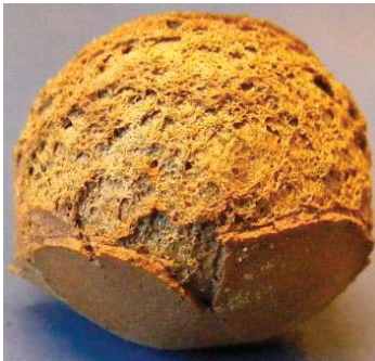
61 62 63 64 65 Caption Fig. 3: Illustration of one pellet of the series lab-16 (16 mm diameter) picturing the heterogeneity of the outer shell. The lower hemisphere exhibits a dense shell; the upper hemisphere exhibits a more porous shell.
