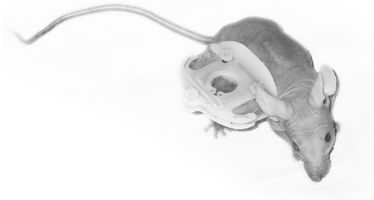
Figure 4. a) Schematic drawing of dorsal window chamber in MRI-compatible material (POM). The hole in the centre is covered by a transparent glass cover slip which is fixed with a clamping ring. The chamber has a total weight of 2.0 g. All parts were produced by the in-house workshop, except for the glass cover slip (Assistent, Germany) b) The MRI-compatible dorsal window chamber implanted in a nude mouse. A circular area is removed from one layer of skin under the glass cover slip, providing a window to the tissue.
