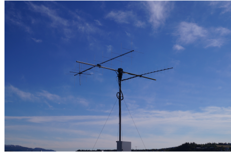
Figure 3.2.: Crossed yagis for 144 MHz and 430 MHz at the Gløshaugen site.
