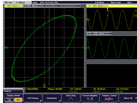
Figure 4.3.: Elliptical shape seen when combining two equal power sinusoids with 45^\circ phase offset in oscilloscope XY-mode.
