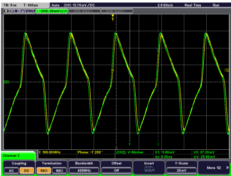
Figure 4.5.: 100 MHz waveform as observed by the oscilloscope.
