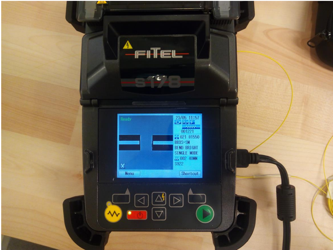
Figure 17 Quality control of fiber tips in Fitel S178 fiber splicer device
