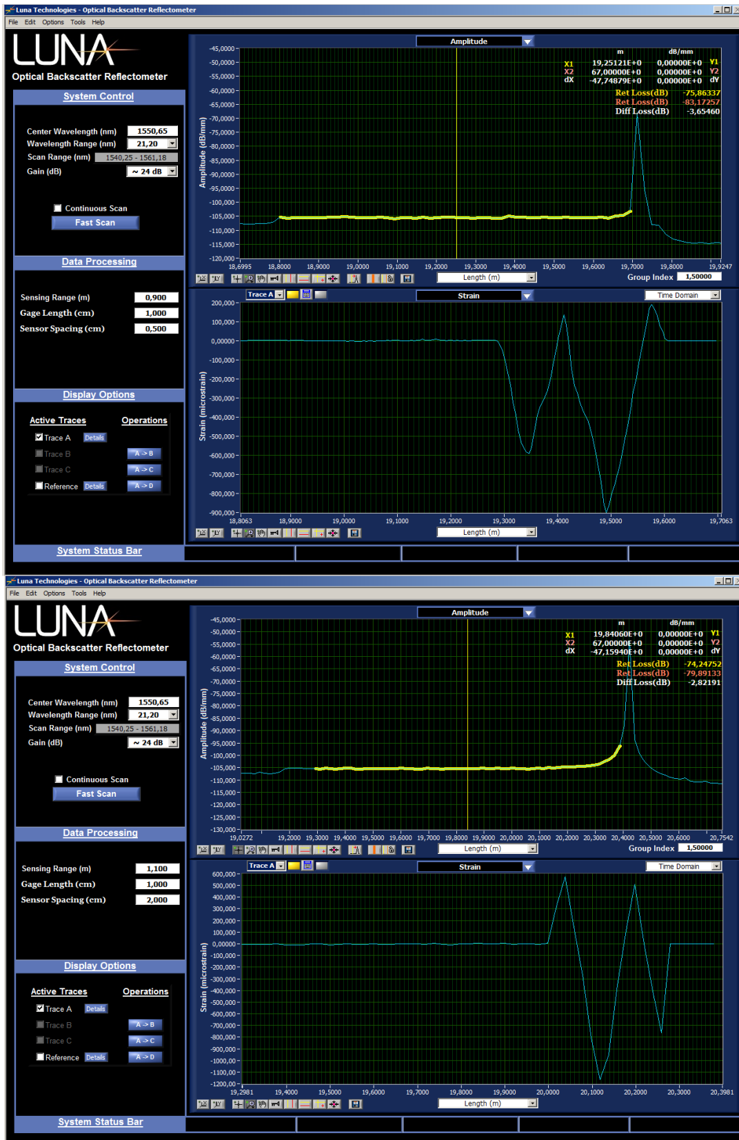
Figure 51 Signals from the second set up of the experimental study with PVC tube at 0 and 90 degrees
