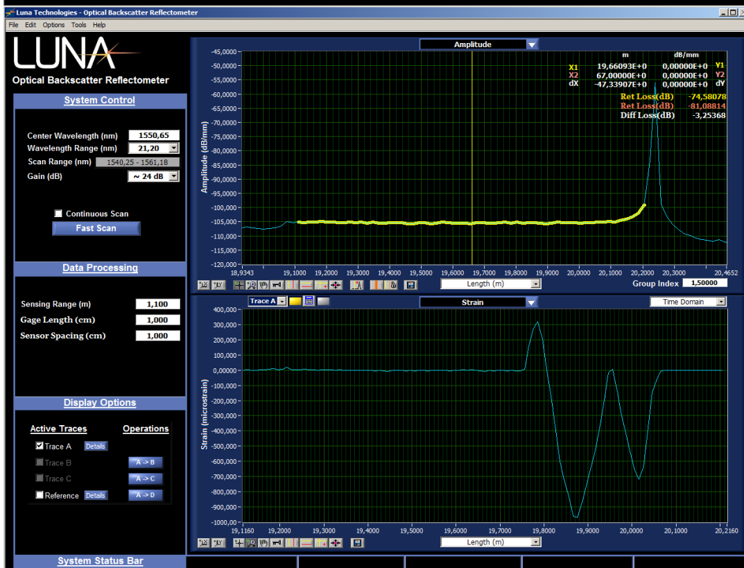
Figure 50 Signals from the first set up of the experimental study with PVC tube at 180 and 270 degrees
