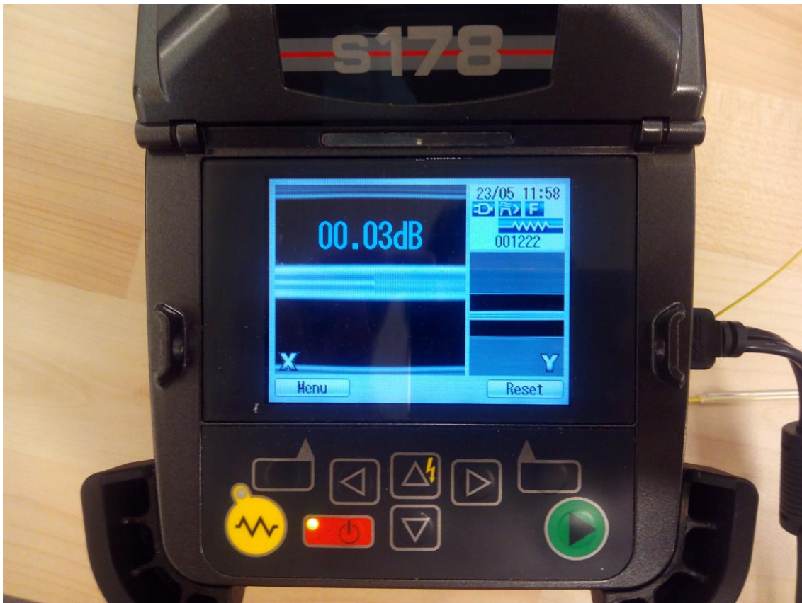
Figure 18 Spliced fibers in Fitel S178 fiber splicer device
