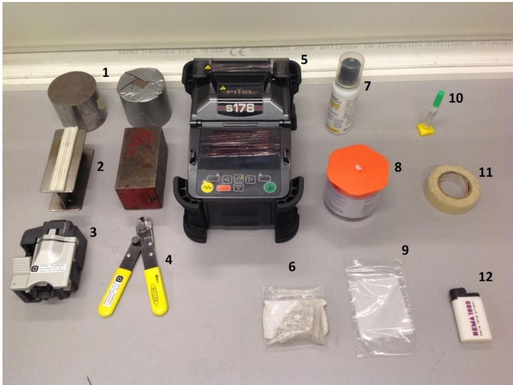
Figure 16 Equipment used for optical fiber splicing
