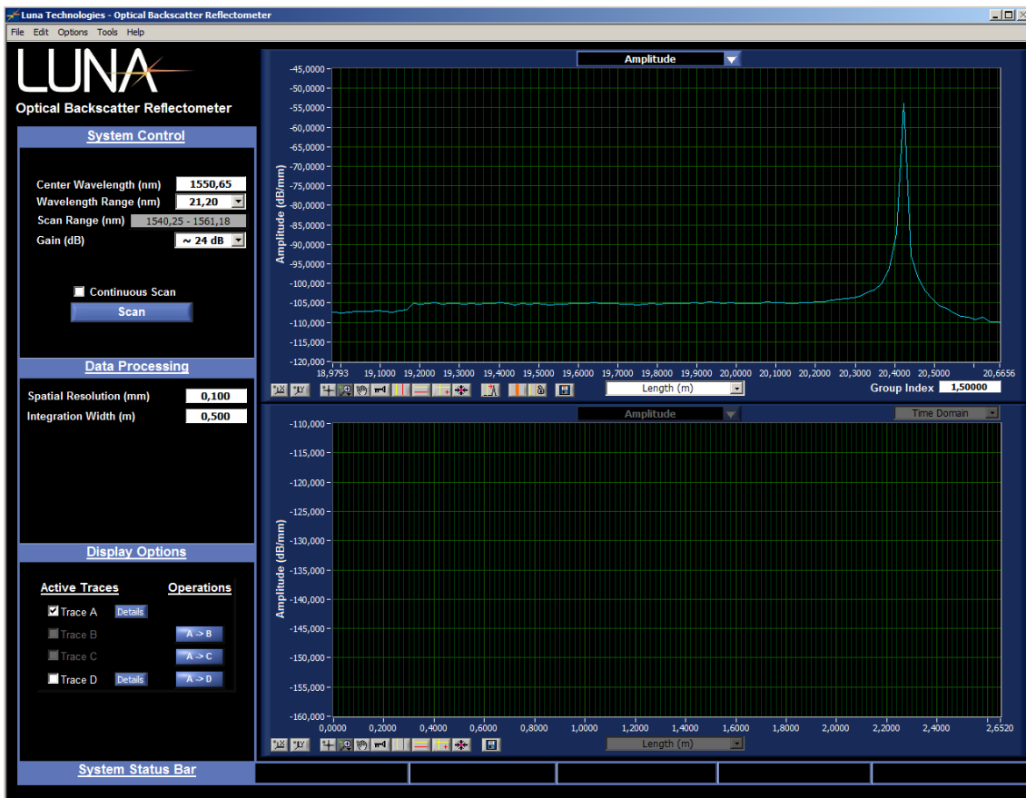
Figure 19 Reference signal from tube through OBR technique
