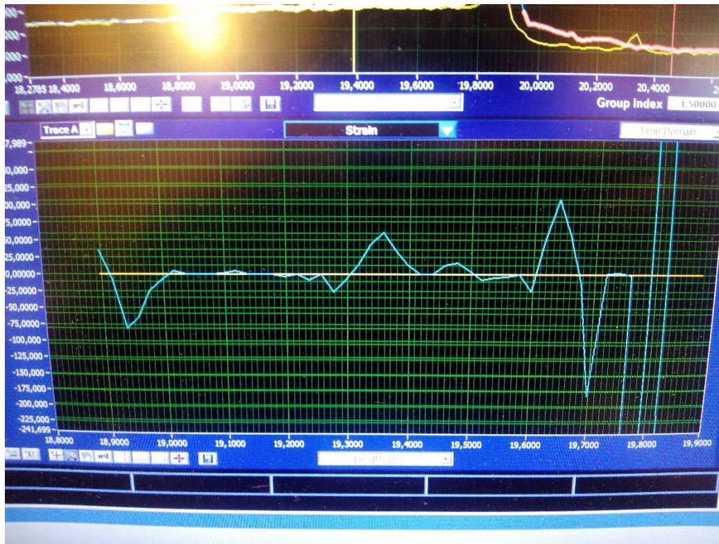
Figure 23 Results of the first adhesion with cyanoacrylate adhesive
