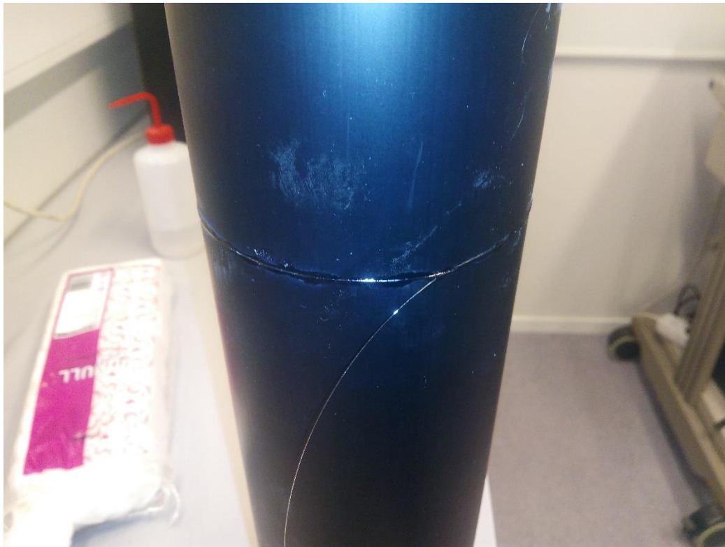
Figure 22 First adhesion done with cyanoacrylate adhesive
