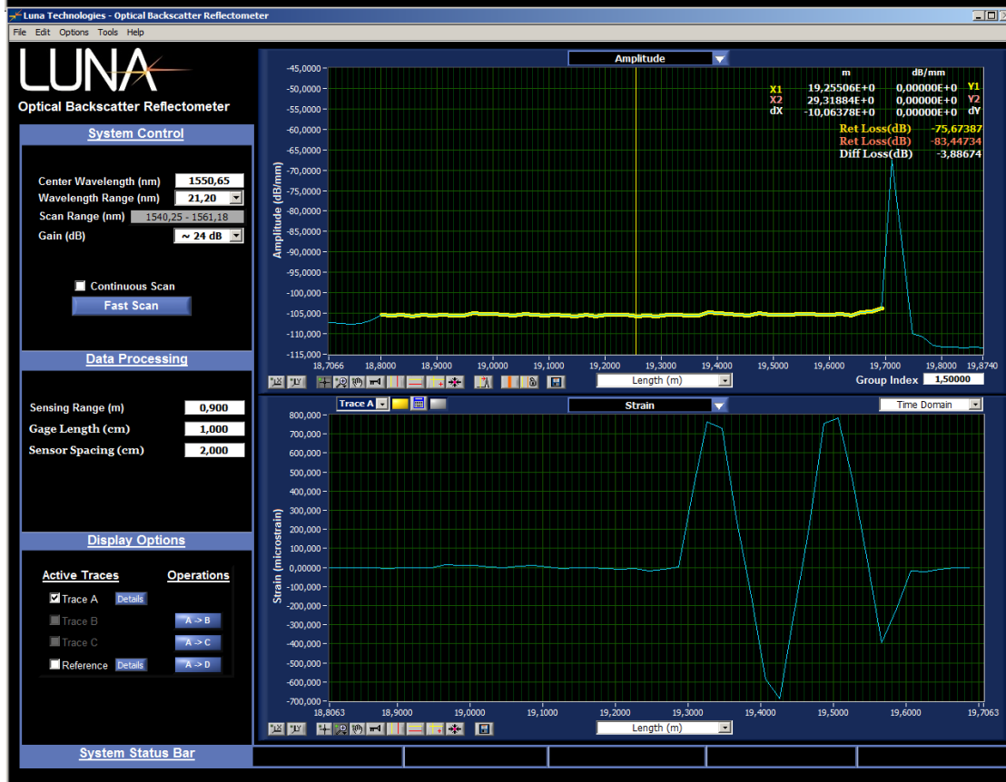
Figure 38 Signals from the second set up of the experimental study with PVC ring at 0 and 90 degrees
