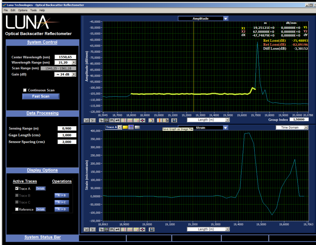
Figure 35 Signals from the first set up of the experimental study with PVC ring at 0 and 90 degrees
