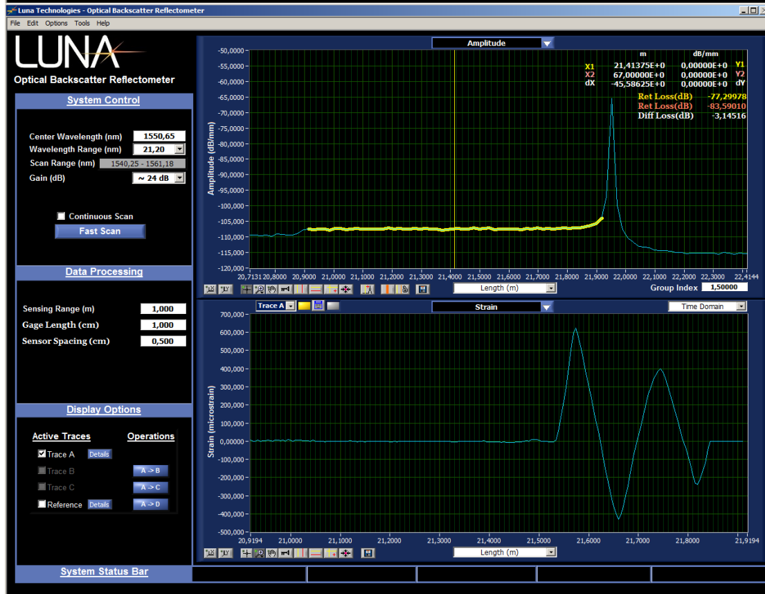
Figure 42 Signals from the third set up of the experimental study with PVC ring at 0 and 90 degrees
