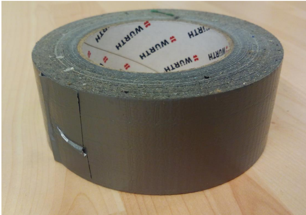
Figure 40 Industrial tape with transverse reinforcements used
