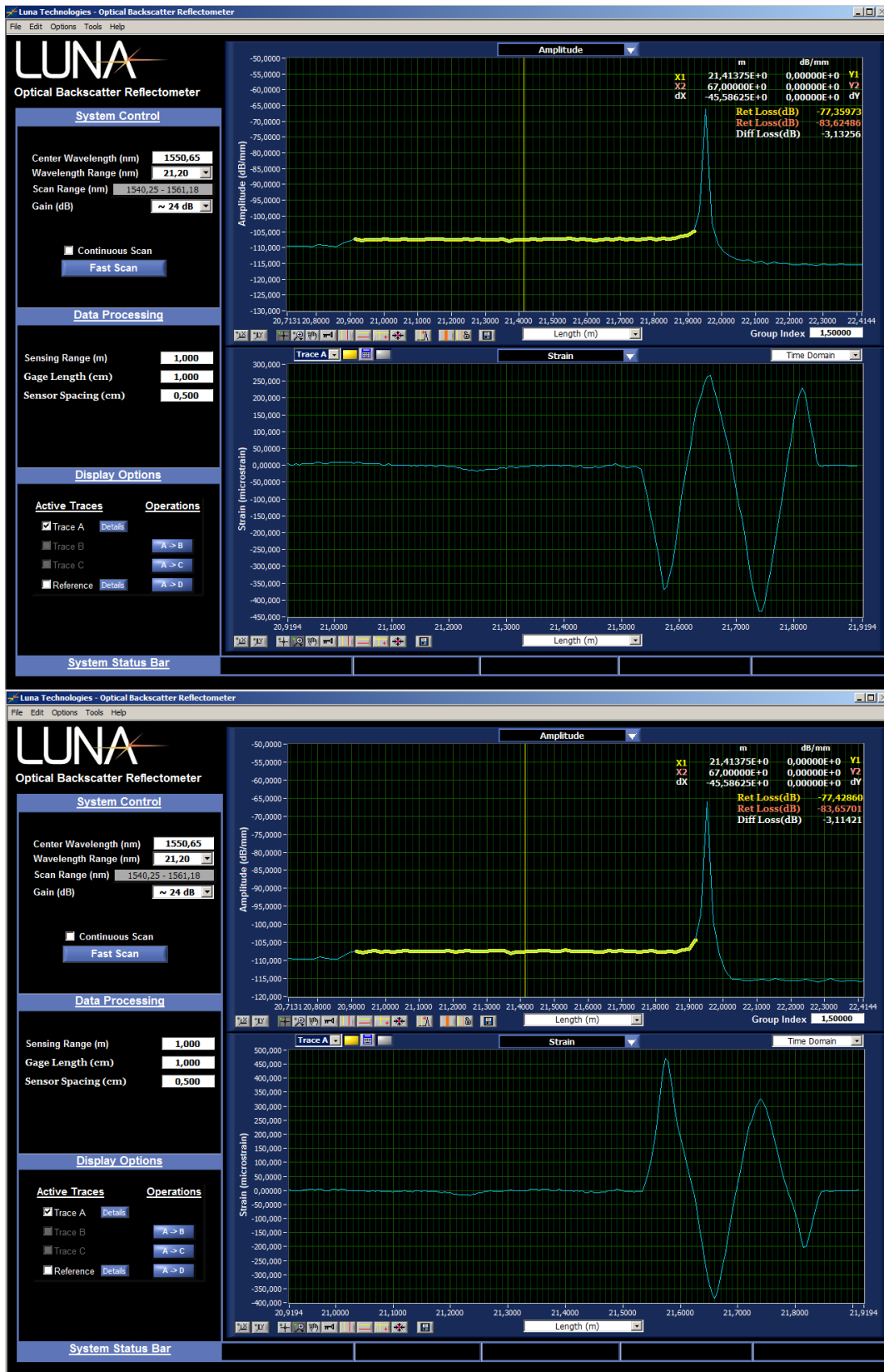
Figure 43 Signals from the third set up of the experimental study with PVC ring at 180 and 270 degrees
