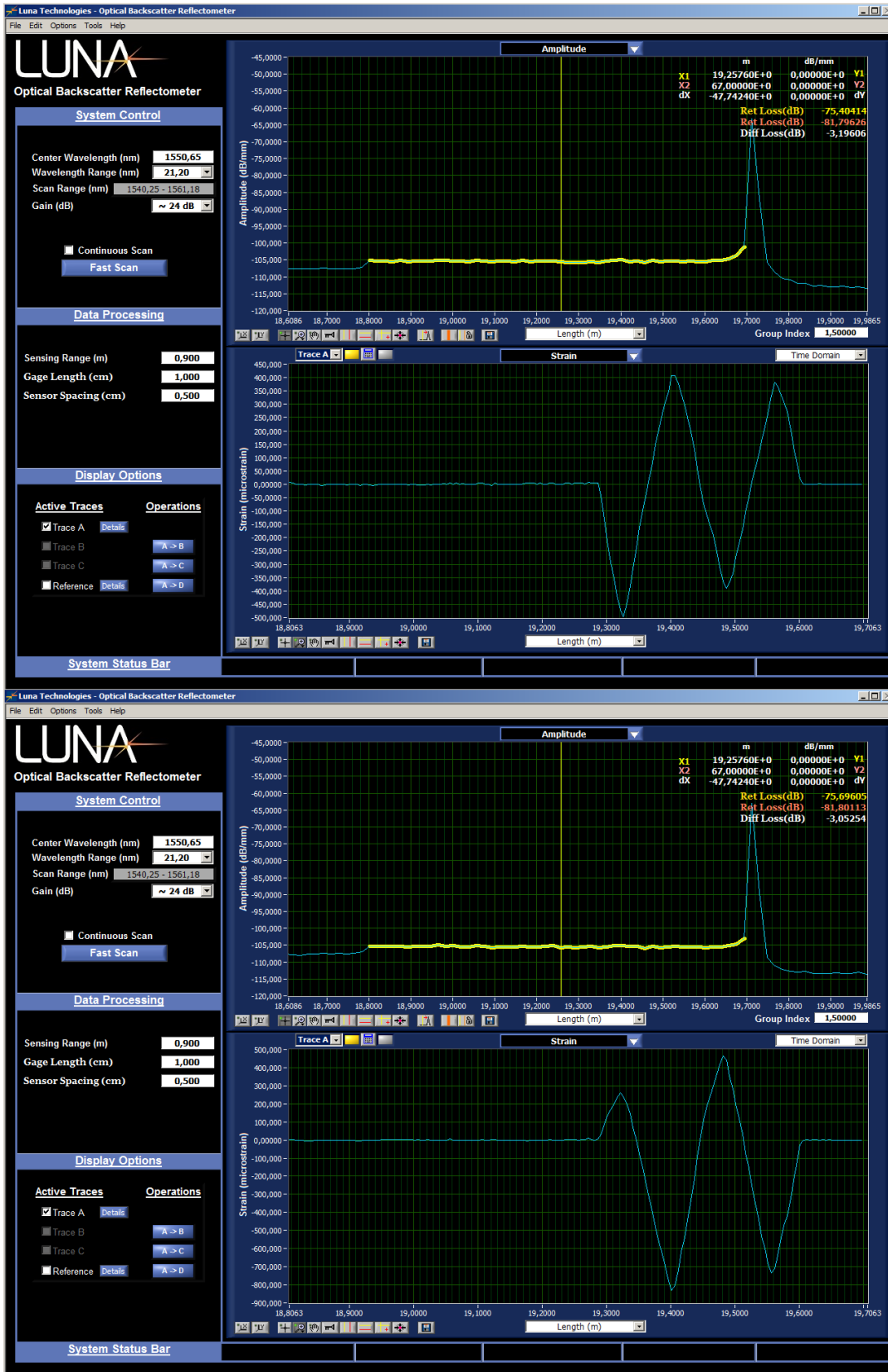
Figure 45 Second signals from the second set up of the experimental study with PVC ring at 180 and 270 degrees
