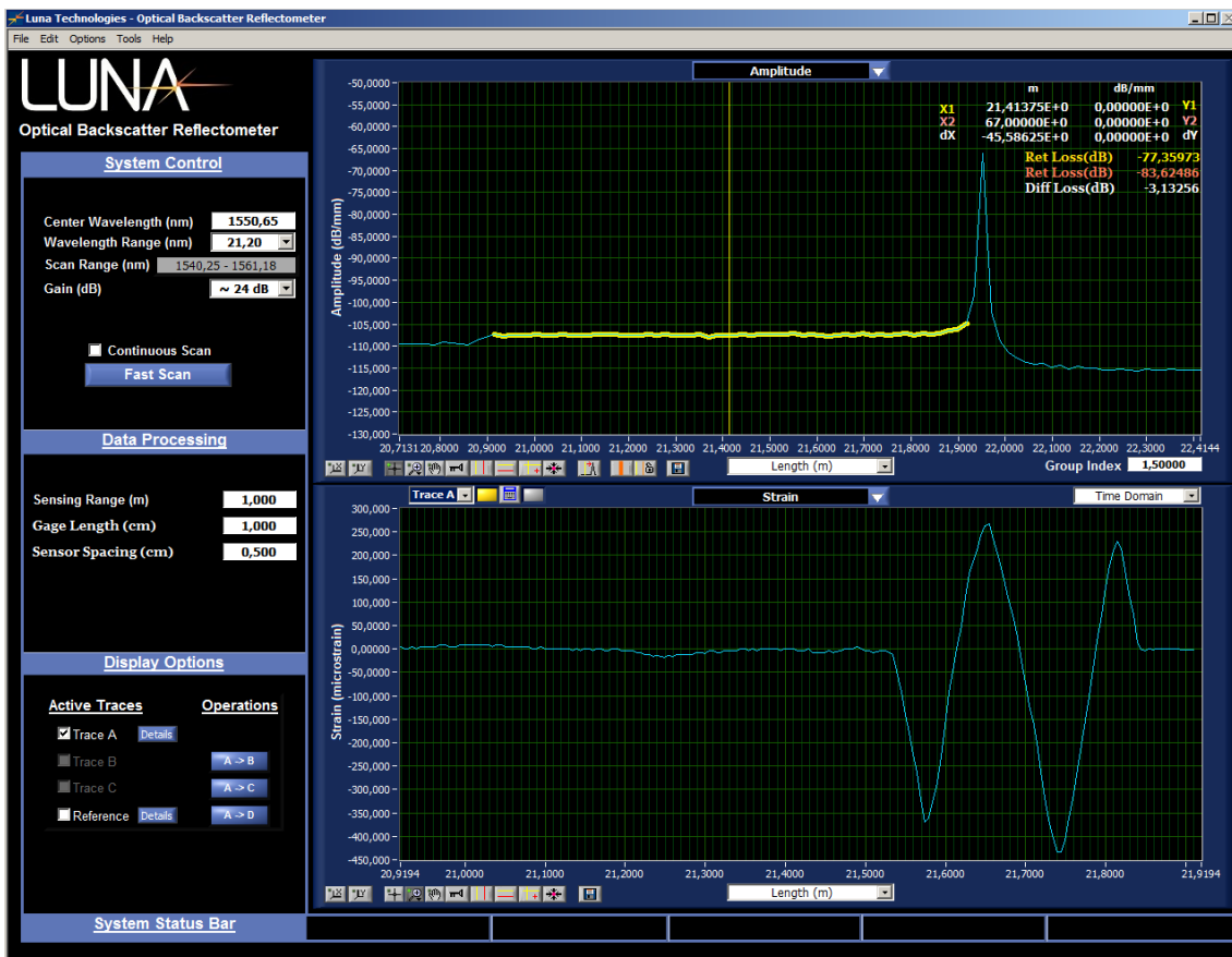
Figure 20 Strain profile signal from tube through OBR technique
