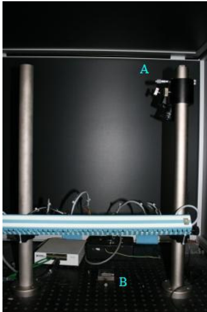
(a) A is the laser which acts as the source for electromagnetic waves. B is where the sample is placed.
