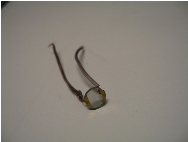
Figure 3.3: The gold covered glass plate which was used as an electrode to apply negative bias over the detector oxide. The gold layer is about 20 nm thick and is therefore transparent.
