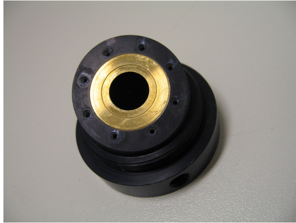
Figure 5.4: The pyroelectric detector with the reflective hemisphere removed.
