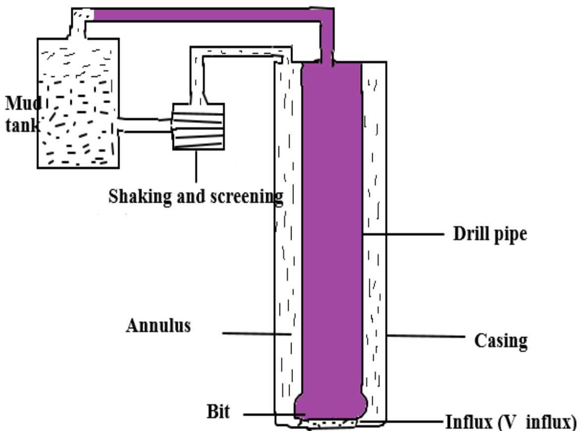
Figure 19: Illustration of increase in volume model
