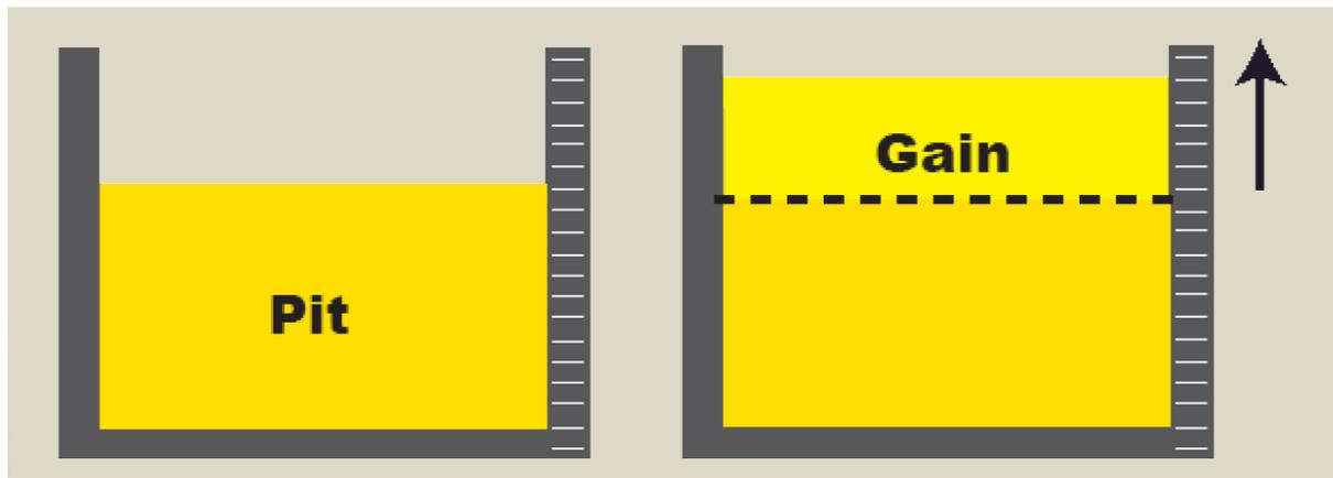
Figure 10: Pit before and after gain
