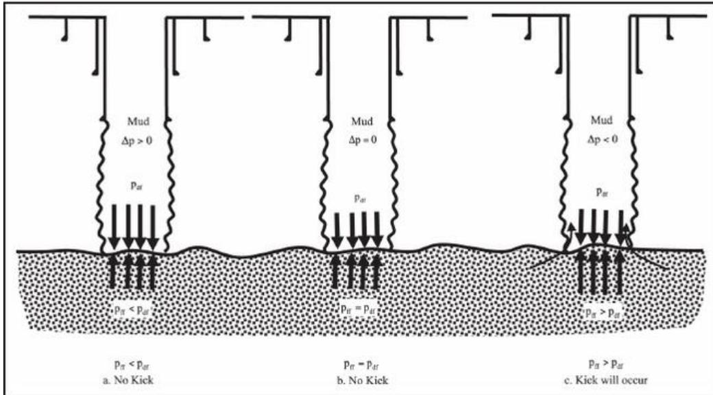
Figure 4: Drilling conditions, a. overbalanced, b. balanced and c. underbalanced.(Azar, 2007)
