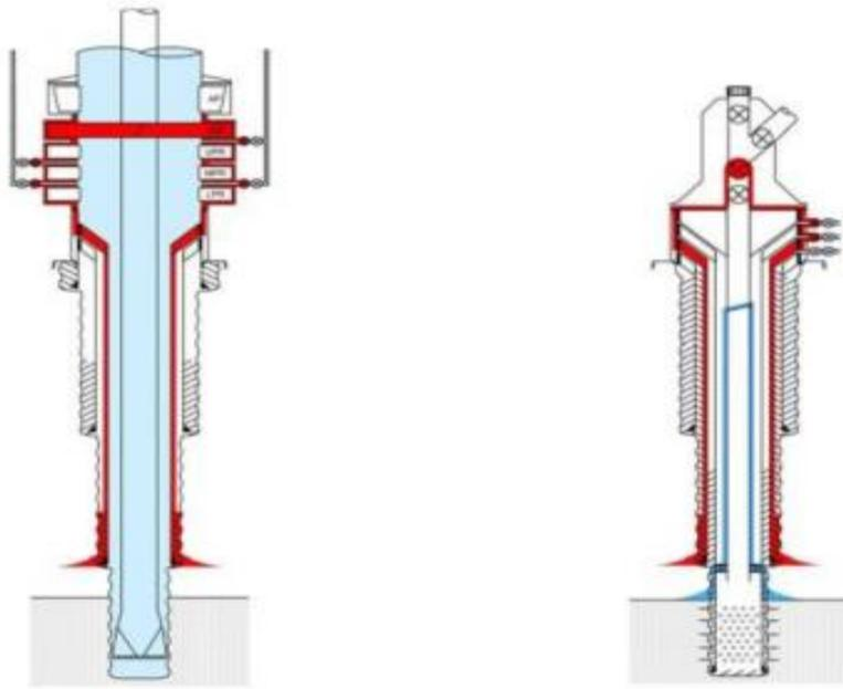
Figure 2: Two barrier envelopes where blue represents primary barrier and red represents secondary barrier(Anders et al., 2015)
