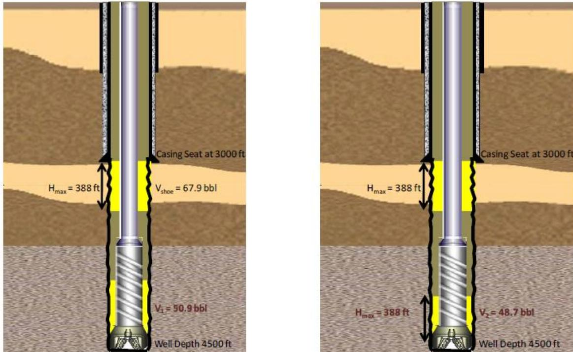
Figure 9: Illustration of  $V_1$  calculation figure on the left, and Illustration of  $V_2$  calculation on the right. (Denney, 2012)
