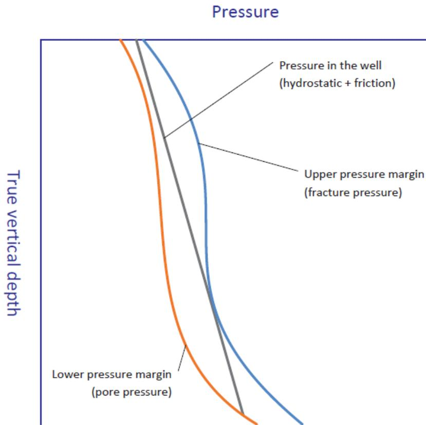
Figure 3: Pore pressure, Hydrostatic pressure and Fracture pressure(Hauge, 2013)
