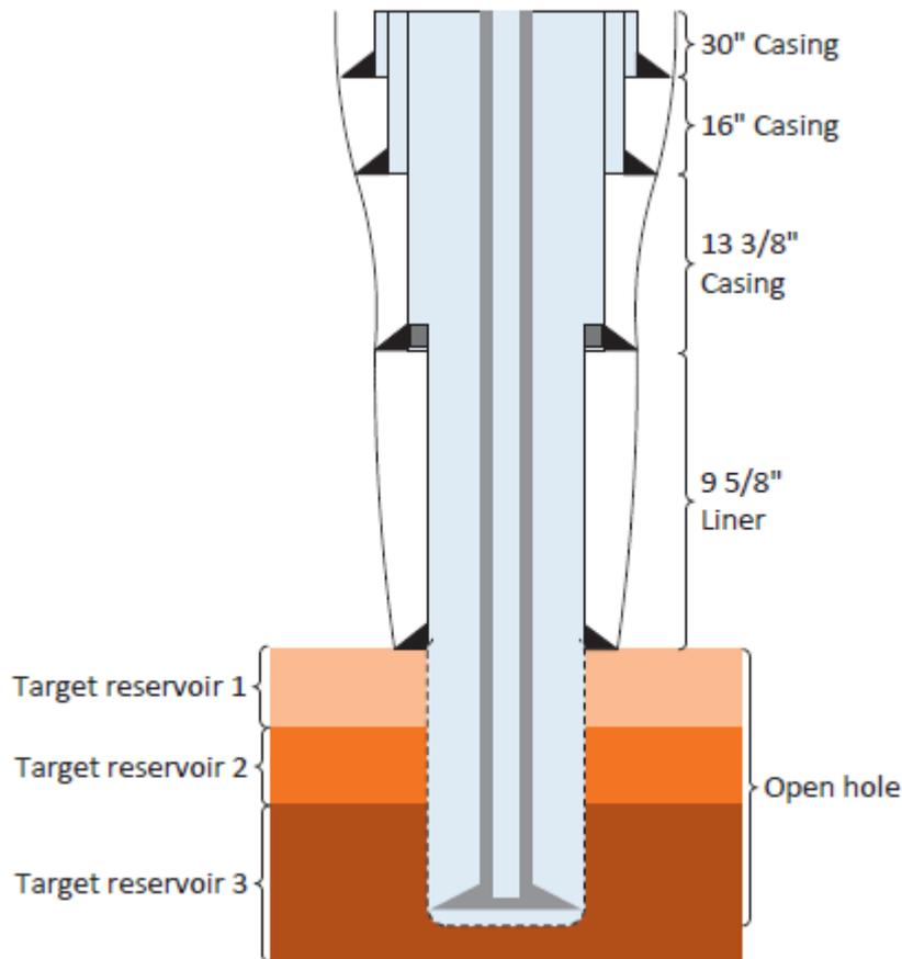
Figure 6: Example of casing program (Hauge, 2013)
