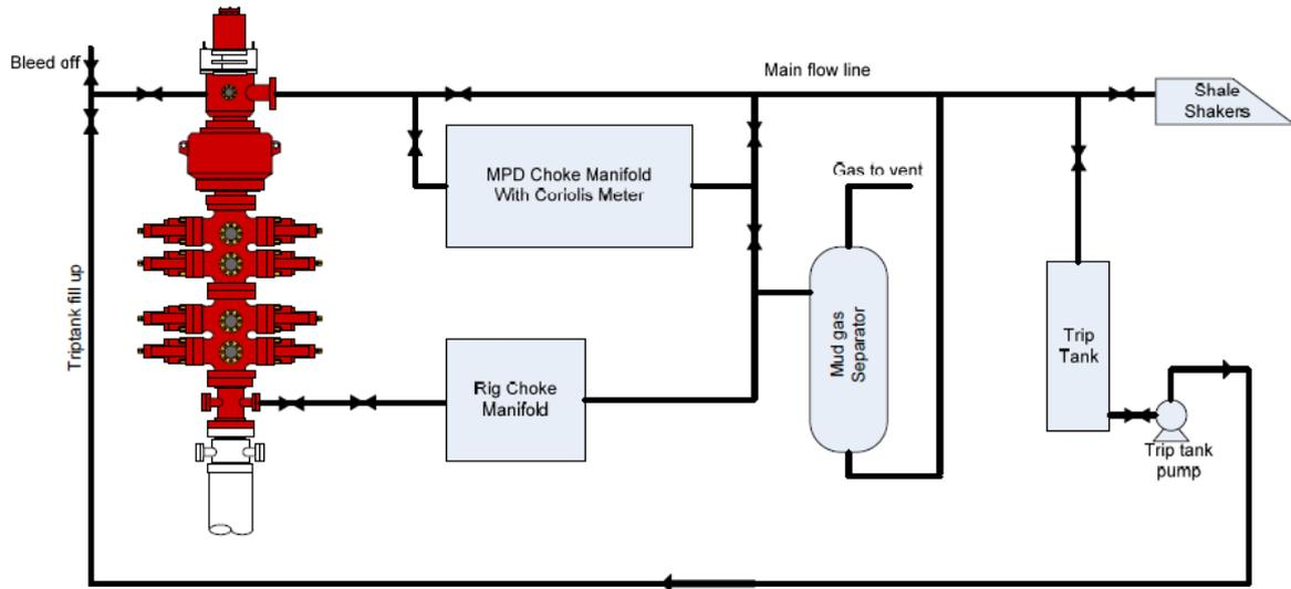
Figure 14: Managed pressure drilling setup in a closed wellbore(Nas, 2011)
