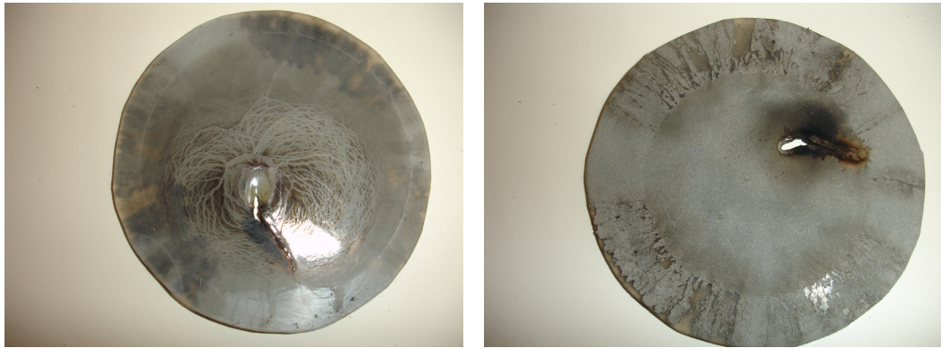
(a) Full picture showing the sample front. (b) The back of the sample also has a large crack going from where it was scorch mark from the breakdown, and var-punctured, and the crack itself is scorched nish has disappeared around the edges. with burning along the edges. The surface is covered in soot, enhancing the traces from the currents going over the edge towards ground.
