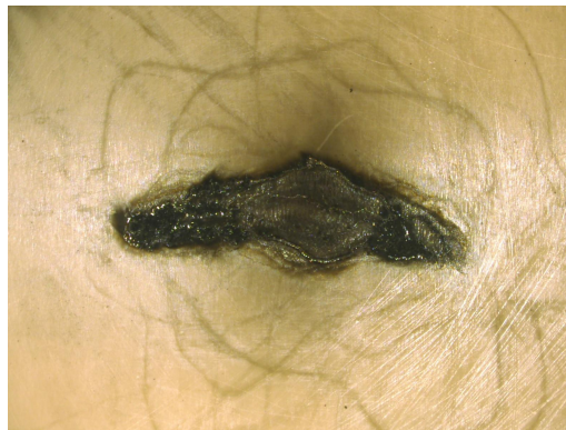
(c) A x8 microscope picture showing a close-up of the puncture in front of the sample. The hole itself is to the far left of the charred area.
