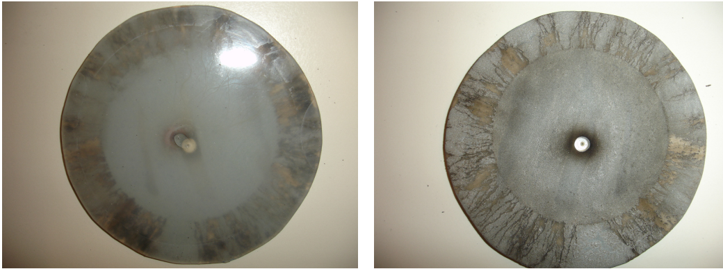
(a) Full picture showing the punctured disc. (b) Picture of the backside showing large The crater and hole is almost circular, and traces in the varnish from charges tracing to- there are no fractures or cracks extending wards ground. from the hole.
