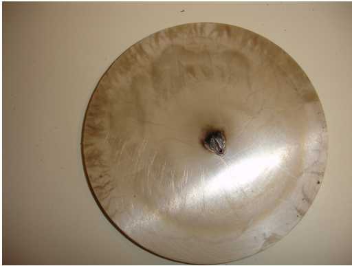
(a) Full picture showing the disc. There is a charred spot near the center, and there are traces of surface charges towards ground as lines going out from the center where surface charges has gone. There also is a flowing pattern in the surface near the edges of the disc. (b) The backside shows much the same a charred spot near the center, and there are traces of surface charges towards ground as lines going out from the center where surface charges has gone. There also is a flowing pattern in the surface near the edges of the disc.
