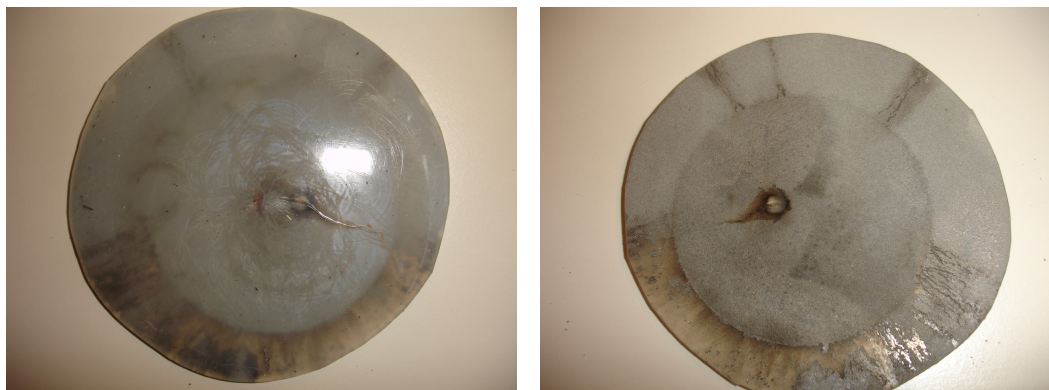
(a) Full picture showing the punctured disc. (b) Picture of the back side. There is a small crater and a crack leading to burnt edges, and the varnish on the lower side is almost removed completely from discharges going around the edge from the front.
