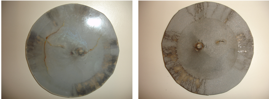
(a) Full picture showing the punctured sample and the large crack moving both to the right and to the left out from the center. (b) Picture of the backside showing large traces in the varnish from charges tracing towards ground.
