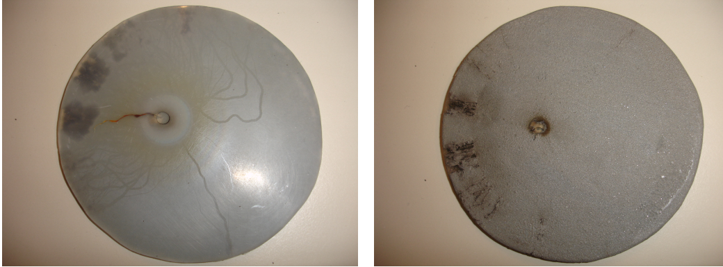
(a) Full picture showing a slightly displaced puncture through the material. The edges around the hole are burnt, and the surface of the material around the hole shows clear signs of currents going out from the center where currents has come around the edge to- and reaching towards the edge of the sample. (b) Full picture showing the backside of the sample. There is a hole in the varnish where the puncture occurred, and traces can be seen in the varnish at the edge of the sample, wards the plane electrode.
