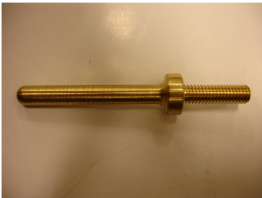
(a) High voltage electrode, 3 mm radius
