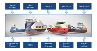
Figure 4.1: Disciplines involved in conceptual phase of Ship Design
