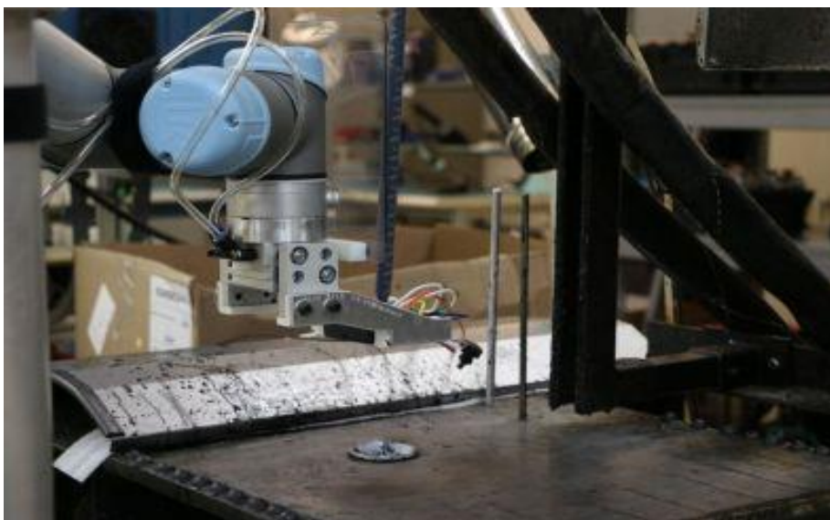
Figure 4-3. Cobot filling epoxy into circuit boards and reduces the risk to human health. (Modern Applications News 2016)
