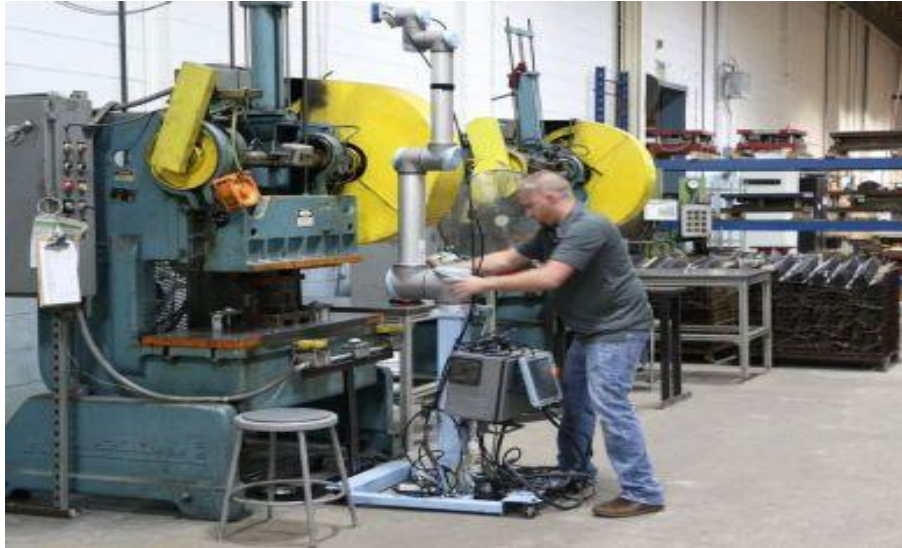
Figure 4-1. The mobile UR10 robot being deployed at a stamping machine in SFEG's sheet metal department. (Modern Applications News 2016)
