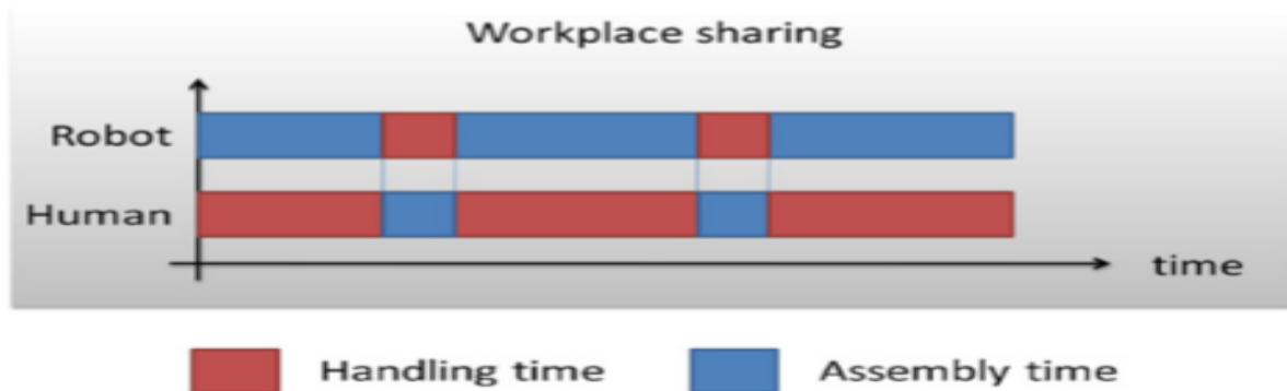
Figure 2-8. Time distribution between human and robot in workplace sharing system. Adopted from (Kruger et al. 2009).
