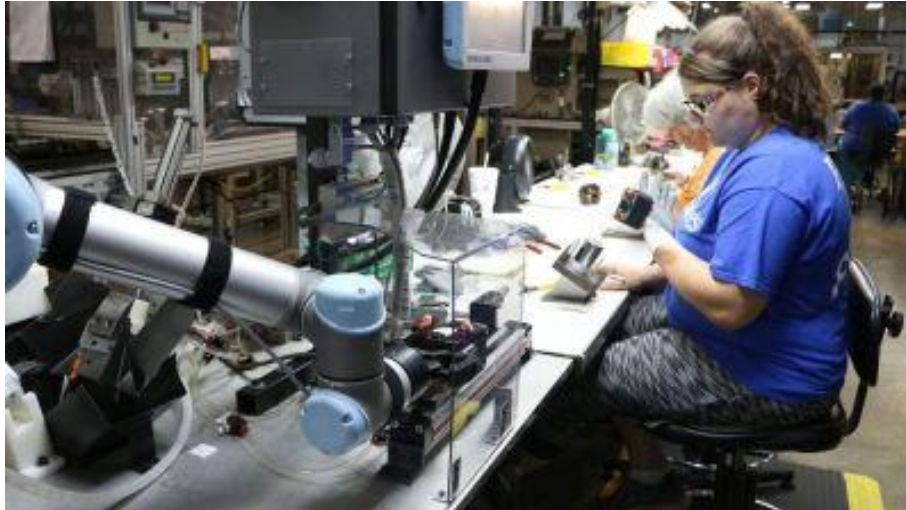
Figure 4-2. UR 5 robot cutting 16000 wires per day. Eliminating the risk of workers to getting carpal tunnel syndrome. (Modern Applications News 2016)
