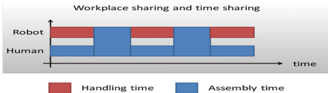
Figure 2-9. Time distribution between human and robot in workplace and time sharing system. Adopted from (Kruger et al. 2009).
