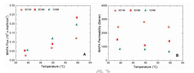
Fig 6 – MAPA flux (A) and permeability (B) obtained from the pervaporation experiments using various DEEA-MAPA blends as a liquid feed at various temperatures.
