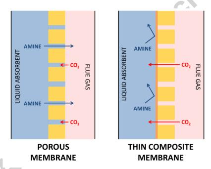
Fig 1 – Membrane contactor schematic representation using porous membranes or thin composite membranes as the interface between the liquid absorbent and flue gas.
