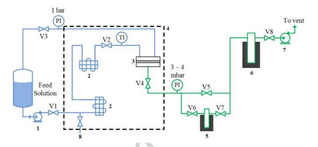
Fig 2 – Pervaporation setup (1: Liquid pump; 2: Heating coil; 3: Membrane module; 4: Heated cabinet; 5: Sampling LN<sub>2</sub> trap; 6: Safety LN<sub>2</sub> trap; 7: Vacuum pump; 8: Liquid purge).
