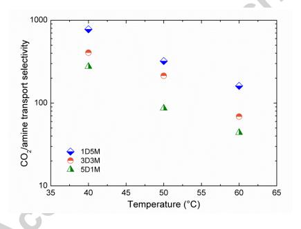
Fig 11 – CO<sub>2</sub>/amine transport selectivity offered by the Teflon AF2400 at various temperatures when DEEA-MAPA blends (1D5M, 3D3M and 5D1M) are considered as liquid absorbents.
