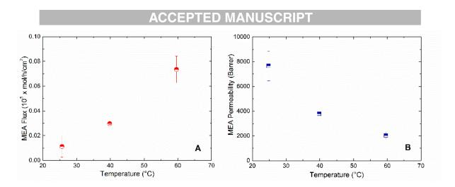
Fig 5 – MEA flux (A) and permeability (B) obtained from pervaporation experiments using 5M MEA as a liquid feed at various temperatures.
