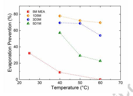
Fig 12 – Evaporation prevention estimated for a non-porous membrane contactor compared to an absorption column for the different absorbents (the dotted lines are intended only to guide the eye).
