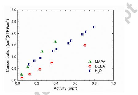
Fig 9 – Uptake of pure H<sub>2</sub>O, DEEA and MAPA in the Teflon AF2400 at 35 °C.
