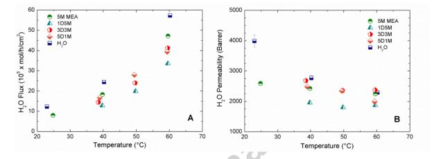
Fig 4 – H<sub>2</sub>O flux (A) and permeability (B) obtained from pervaporation experiments for pure H<sub>2</sub>O and various absorbents (5M MEA, 1D5M, 3D3M and 5D1M) at different temperatures.
