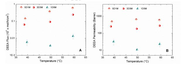
Fig 7 – DEEA flux (A) and permeability (B) obtained from the pervaporation experiments using various DEEA-MAPA blends as a liquid feed at various temperatures.
