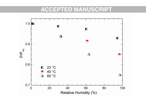
Fig 8 – Relative variation of  $CO_2$  permeability at different RH compared to the dry value ( $P_{dry}$ ). For the numerical values refer to Table 2.
