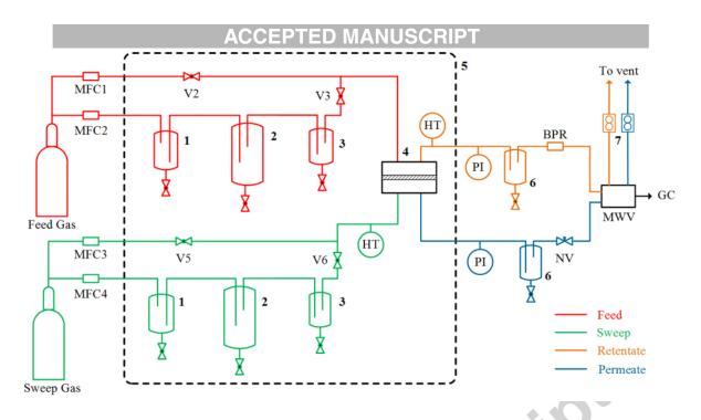
Fig 3 – Mixed gas permeation rig (1: MFC-safety trap; 2: Humidifier; 3: Droplet trap; 4: Membrane module; 5: Heated cabinet; 6: Water knockout; 7: Bubble flowmeters; MFC: mass flow controller; NV: Needle valve; BPR: Back pressure regulator; PI: Pressure indicator; HT: Humidity and temperature sensor; MWV: Multi-way valve; GC: Gas chromatograph).
