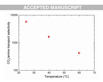
Fig 10 – CO<sub>2</sub>/amine transport selectivity offered by the Teflon AF2400 at various temperatures when 5M MEA is considered as a liquid absorbent.
