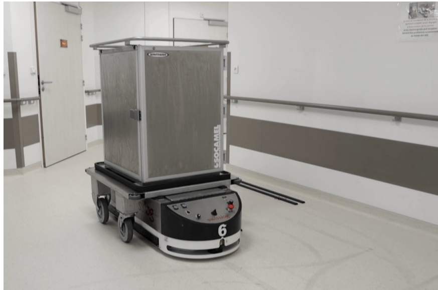
Fig. 3.2: AGV robot carrying a container of supplies at St. Olavs Hospital. (St Olavs, 2017) [22]
