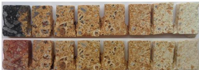
**Figure 6. Samples before (upper) and after (lower) heat treatment. The samples closest to the anode side were clearly blackened during operation in the anode baking furnace.**
