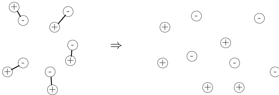
Figure 3.3: In the two dimensional Coulomb gas, dipoles unbind in a Berezinskii–Kosterlitz–Thouless phase transition to form a metallic plasma.
