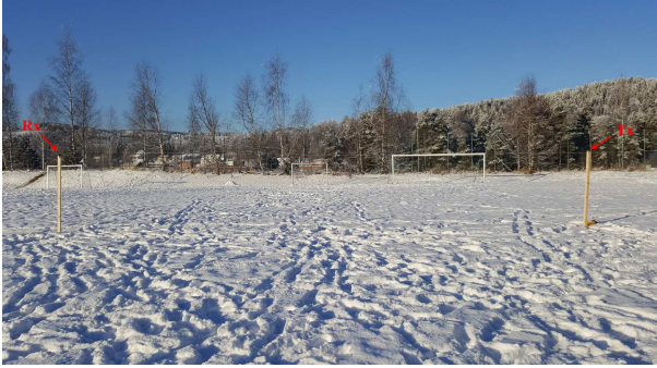
Fig. 2. Measurement site: a large football field covered by snow with Tx and Rx nodes mounted on a mass of different heights (0.25 m, 1 m and 1.5 m) from the ground.
